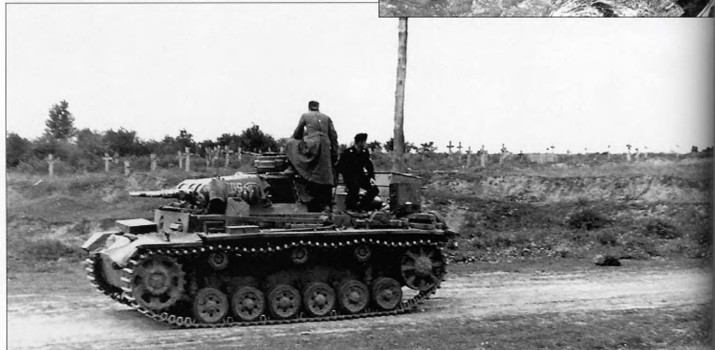
An early Pz.Bef.Wg.III Ausf.H fitted with the early 3.7cm dummy gun and, unusually, a later cast drive sprocket. Evidence of past battles can be seen in the rows of crosses on the graves of fallen German soldiers in the background.
