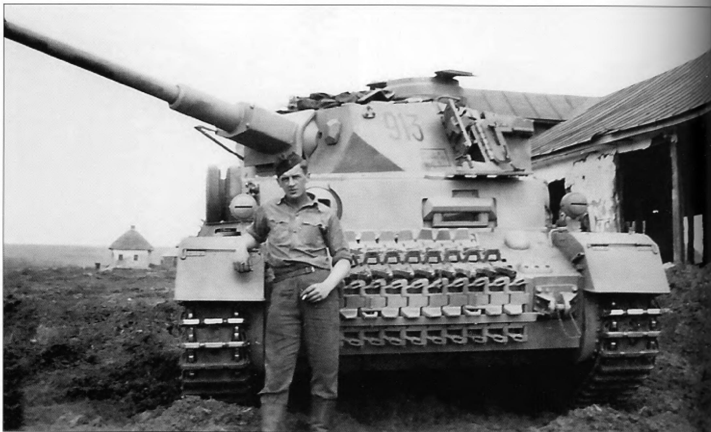
The 30mm Zusatzpanzer and antenna deflector can be clearly seen on this new Pz.Kpfw.IV Ausf.G seen in Russia in the summer of 1942. Unusually, a shipping stencil can be seen painted on the lower front side of the turret. The light color suggests that it is also painted in a tropical scheme. The final drives on the Ausf.A to Ausf.G were protected with curved armor plates bolted to the housing which can be clearly seen in this photo. Reinforced final drive housings were introduced on the Ausf.H which eliminated the curved plates.
