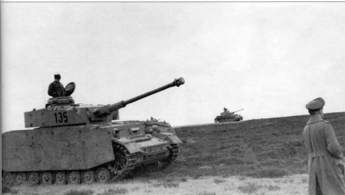
Another Pz.Kpfw.IV Ausf.H from the same unit displaying a complete set of early hull Schürzen modified to fit the new rail system.
