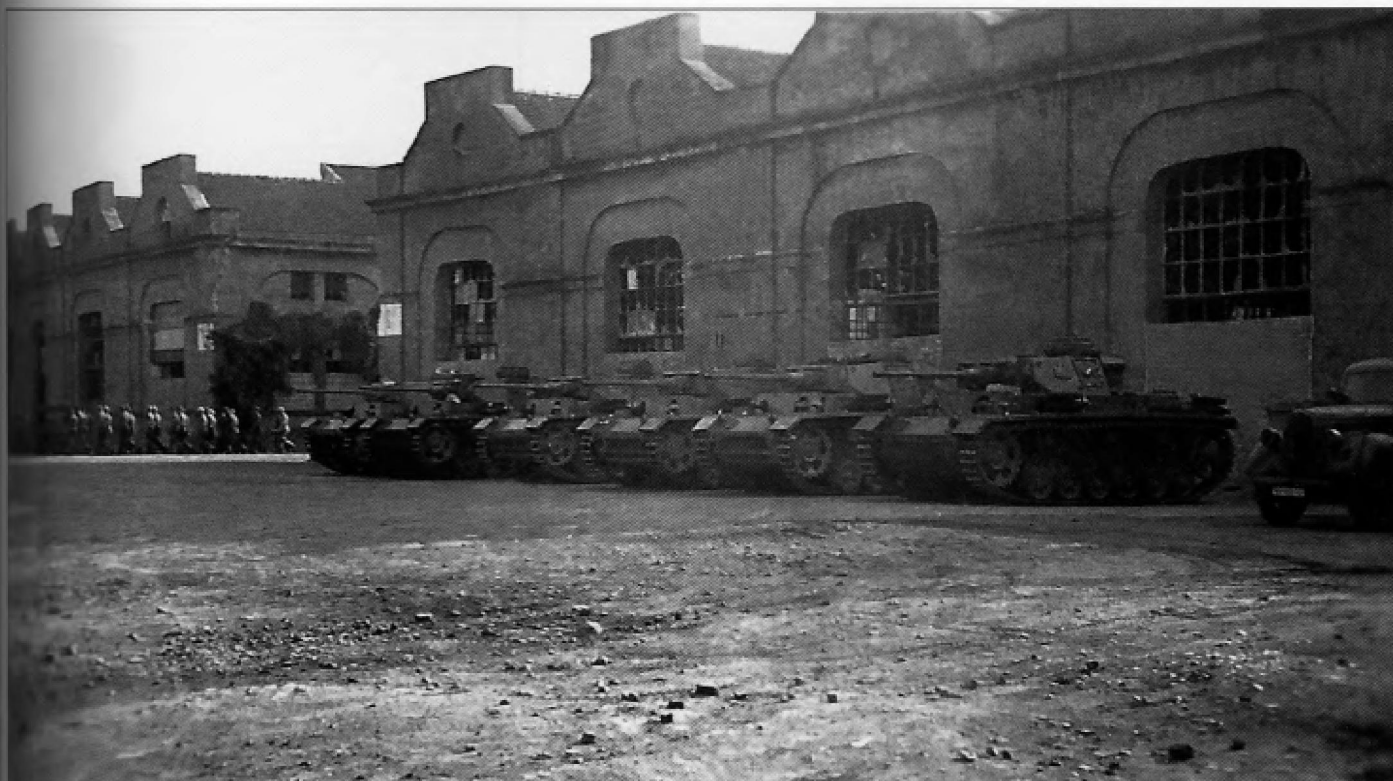
A mixed group of Pz.Kpfw.III Ausf.J and L sit in front of a workshop building, probably somewhere in Germany. None of the vehicles has had the 30mm armor plate installed on the mantlet. The turret side visor can be seen on the nearest vehicle but not on the remainder.
