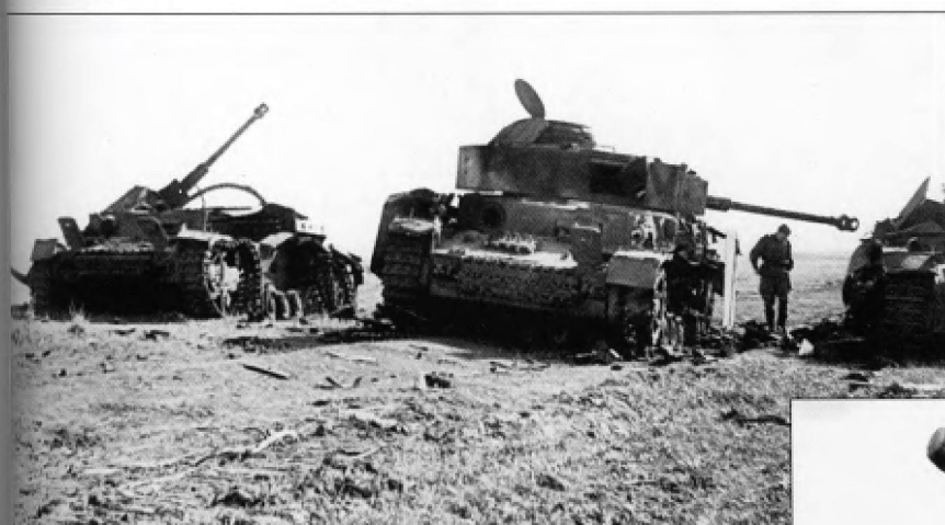
The early style of hull Schürzen was attached using hooks welded to a steel angle frame that ran down the side of the hull with additional hooks bolted to the fenders. Holes were cut into the plates for the hooks to go through. This arrangement often resulted in damage or loss of the skirts when snagged on brush and was changed to a saw-toothed early during production of the Ausf.H. A shipping stencil can be seen painted on the Schürzen just in front of the white outline Balkenkreuz.
