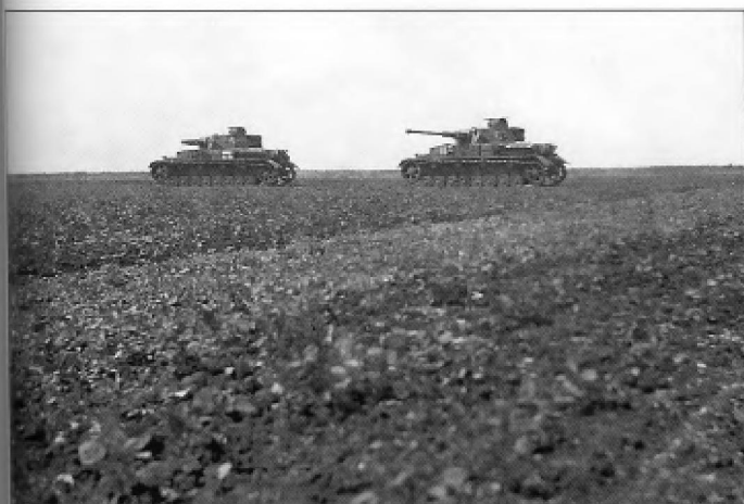
A Pz.Kpfw.IV Ausf.F and a Pz.Kpfw.IV Ausf.F2 from Pz.Abt. 'Großdeutschland' photographed on the Eastern Front during the summer of 1942. This photo provides a good comparison of the difference between the short and long barrel Pz.Kpfw.IV.
