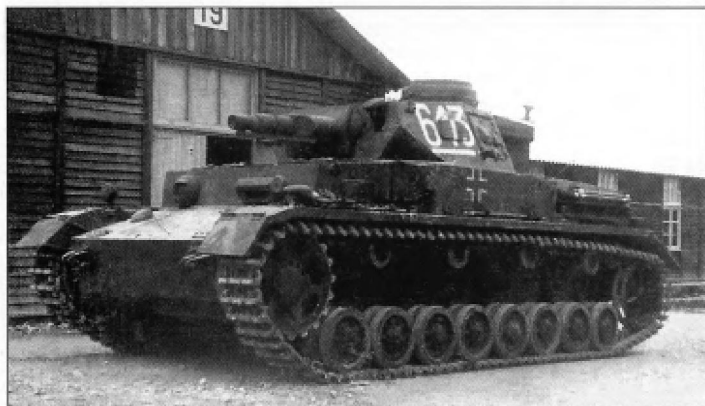
An armored brake cooling vent was added to the brake access hatches on the glacis. The new drive sprocket and idler design along with the two-piece turret side hatches can be seen in this photo. Other improvements include a new shorter muffler, modifying the turret traverse motor muffler and redesigning and moving the armored smoke candle rack to the left side of the rear plate. There were 462 Pz.Kpfw.IV Ausf.F produced from April 1941 to March 1942.
