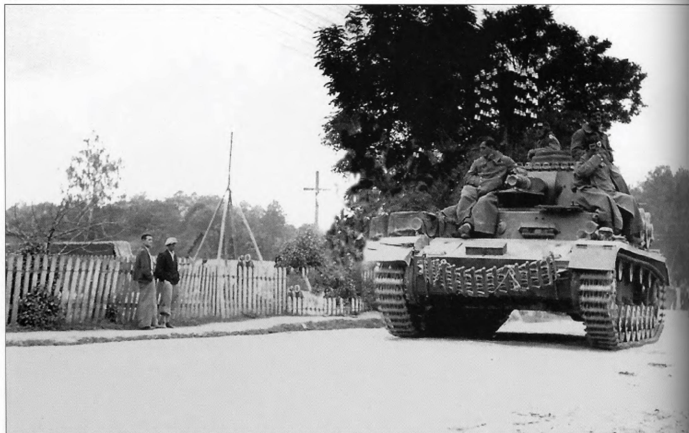
This Pz.Kpfw.IV Ausf.E is one of the early production vehicles that did not receive the additional 30mm armor plates on the front and sides of the superstructure. New flush steering brake access hatches were also introduced on Ausf.E production. The tactical emblem for 9.Panzer-Division can be seen painted to the left of the driver's hatch.
