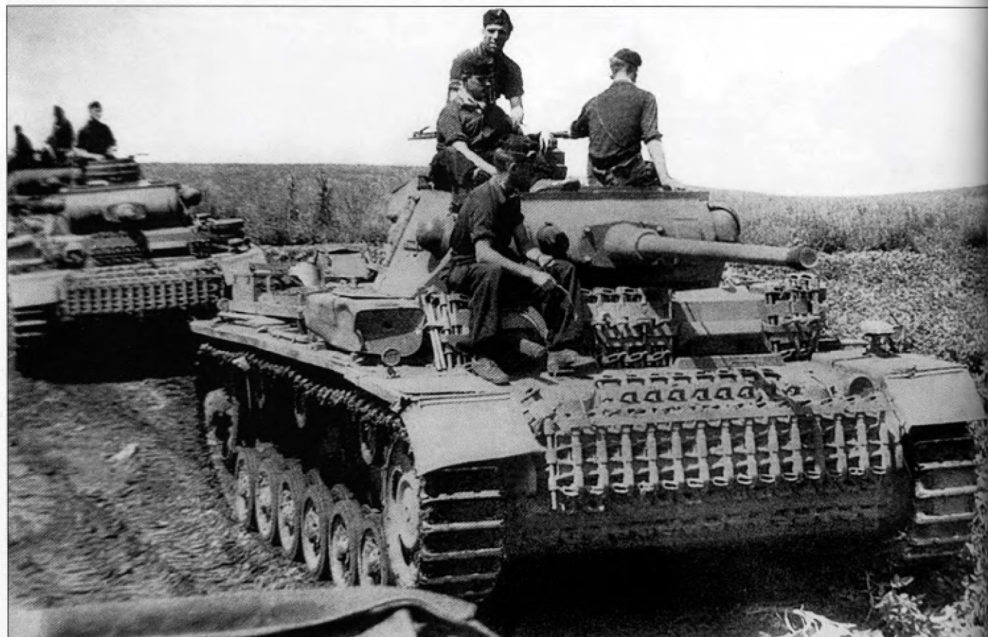
The Pz.Kpfw.III Ausf.J with the 5cm KwK L/60 gun was brought into service in early 1942, but was still not powerful enough to effectively deal with the Russian T-34 or KV tanks. Due to the longer ammunition, the amount that could be carried was reduced to 84 rounds.
