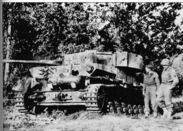
Another Pz.Kpfw.IV Ausf.H from the same unit displaying a complete set of early hull Schürzen modified to fit the new rail system.
