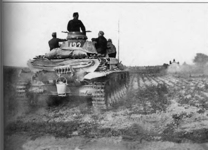
The steep slope of the engine ventilation grilles can be seen in this rear view of a Pz.Kpfw.IV Ausf.B or C. The Pz.Kpfw.IV Ausf.A to F were fitted with flat engine deck hatches, with the exception of those Ausf.D to F that were tropicalized, so stowage piled on the engine deck did not present a problem. This vehicle is missing the small, horizontal turret traverse motor muffler normally fitted above the main exhaust muffler.
