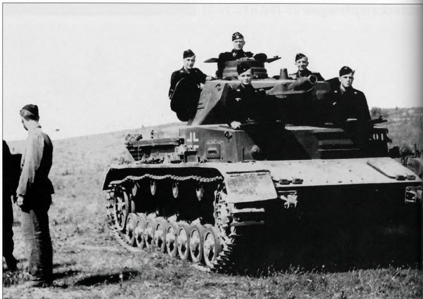
This Pz.Kpfw.IV Ausf.B or C is seen in France in the spring of 1940. Note the new style of Balkenkreuz that replaced the highly visible larger white crosses that were previously used. Unfortunately, the radio operator standing in his hatch is hiding the coaxial MG, the most prominent feature that could positively identify this as an Ausf.B or C. The number '201' can be seen painted beside the driver's visor.
