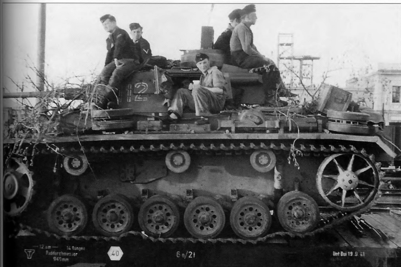
The crewmen of this new Pz.Kpfw.III Ausf.J, armed with the 5cm KwK L/60 gun, are enjoying a relaxing ride to the front on a railcar bound for the Russian Front. Beginning with Ausf.J production, two spare road wheels were stowed on special mounts on the left fender.
