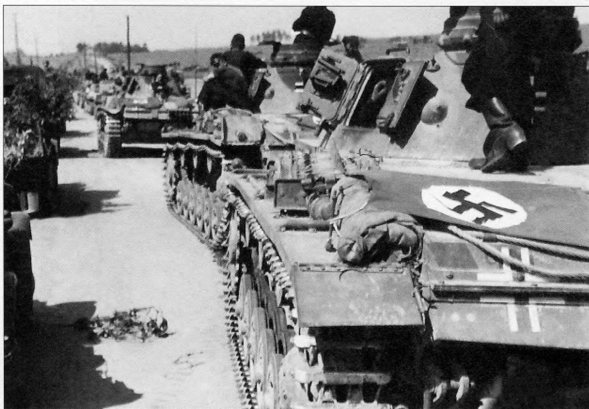
This battered Pz.Kpfw.III Ausf.E or F is being transported to a repair depot on an Sd.Ah.116 trailer after the battle of France in 1940. Due to overlapping production schedules and the presence or absence of certain external features, it is often impossible to accurately determine the specific model, or Ausf. of the vehicle. In such cases, the chassis number is the only accurate way to tell. This vehicle displays features common with some Ausf.E and F such as the radio operator's visor, but lacks the splash strip in front of the turret and the armored vents for brake cooling on the glacis that were introduced during Ausf.F production. After the Polish campaign, the German Army adopted a less conspicuous, smaller black Balkenkreuz with a white outline to mark their armored vehicles. It is most likely painted in the two color camouflage scheme of 2/3 dunkelgrau Nr.46 and 1/3 dunkelbraun Nr.45 ordered for armored vehicles on 7 November 1938, largely obscured by a heavy coat of dust.
