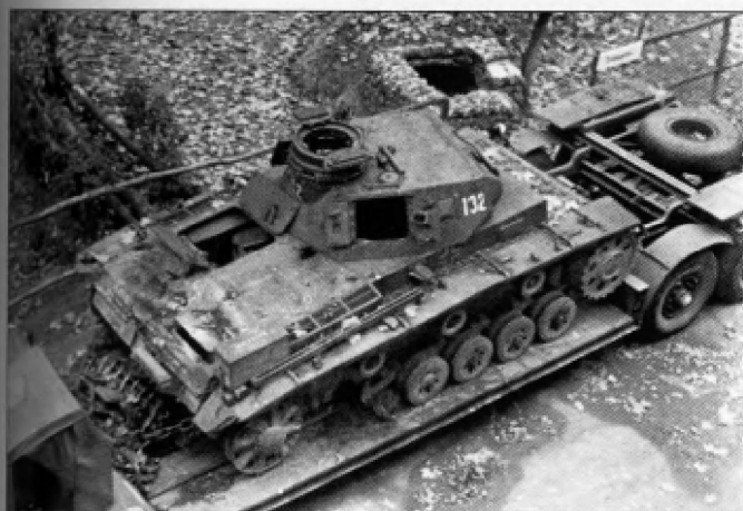
A Pz.Kpfw.III Ausf.E seen early in the Polish campaign, boldly marked with a large white Balkenkreuz on the front plate. The chassis number '60408' can be faintly seen on the front glacis plate making this the eighth Ausf.E produced. A hit on the front of the turret has torn away the right side of the external gun mantlet and made a small penetration hole in the 30mm armor plate. There were 96 Pz.Kpfw.III Ausf.E produced from December 1938 to October 1939.
