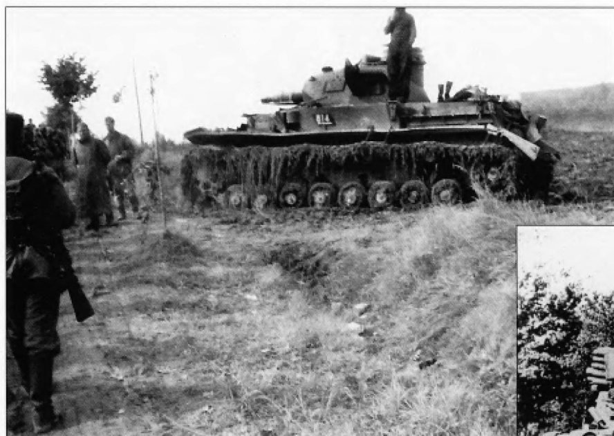
This is a Pz.Kpfw.IV Ausf.D that was converted to a Tauchpanzer and assigned to Pz.Rgt.18 of the 18.Panzer-Division seen in Russia in 1941. It is towing a special fuel trailer. The standard muffler was replaced with a deep wading exhaust system which can be seen on the rear of the hull. During the early successes when the Panzers advanced with lightning speed, it was common practice to display the Nazi flag to identify German tanks to Luftwaffe pilots from the air.
