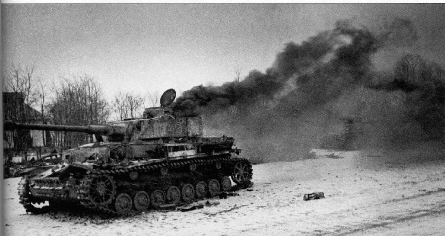
A Pz.Kpfw.IV Ausf.H burns furiously during the winter of 1943-44 somewhere on the Russian Front. A new cast drive sprocket and reinforced final drive housing was introduced on Ausf.H production starting in April 1943. The early style road wheel hubs and rubber tired return rollers identify this vehicle as being produced sometime before September 1943.
