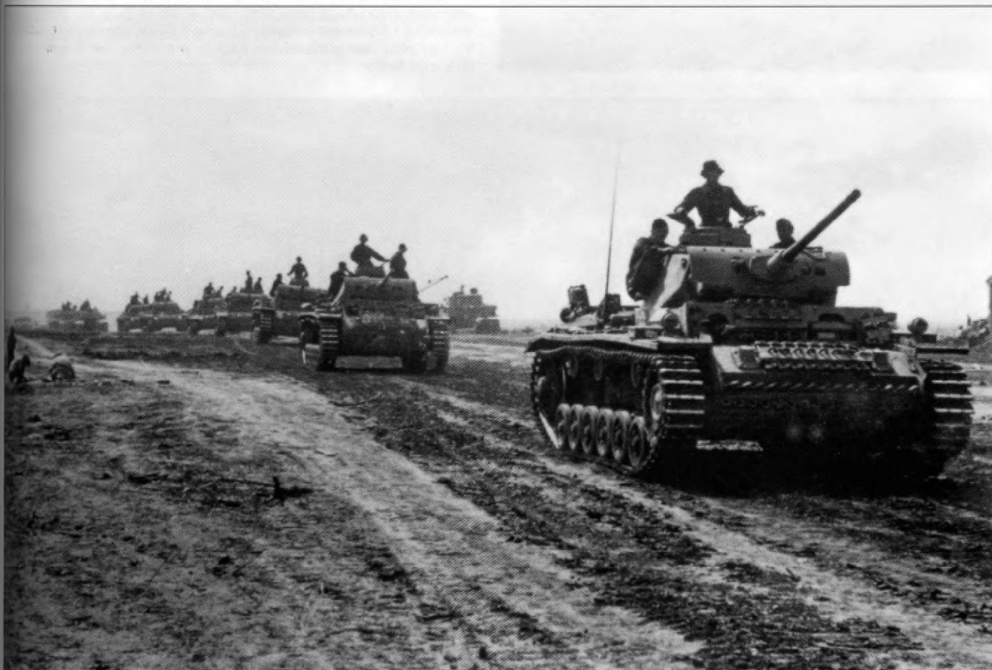
Beginning with the Pz.Kpfw.III Ausf.M, two Bosch headlights were installed on the left and right fenders in place of the lights previously installed beside the armored brake cooling vents on the glacis. Here we see the 30mm armor plate installed on the mantlet in addition to the spaced 30mm plate on the front of the superstructure.
