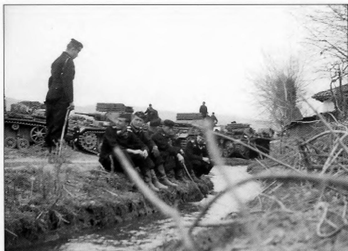
A mixed column of Pz.Kpfw.III's has halted along a small stream and the crews are taking a short break. The vehicle on the left is a Pz.Kpfw.III Ausf.H and is fitted with the new idler wheel. Although not clearly evident here, the turret design has been modified to incorporate a single piece rear plate.
