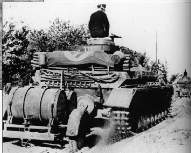
This is a Pz.Kpfw.IV Ausf.D that was converted to a Tauchpanzer and assigned to Pz.Rgt.18 of the 18.Panzer-Division seen in Russia in 1941. It is towing a special fuel trailer. The standard muffler was replaced with a deep wading exhaust system which can be seen on the rear of the hull. During the early successes when the Panzers advanced with lightning speed, it was common practice to display the Nazi flag to identify German tanks to Luftwaffe pilots from the air.
