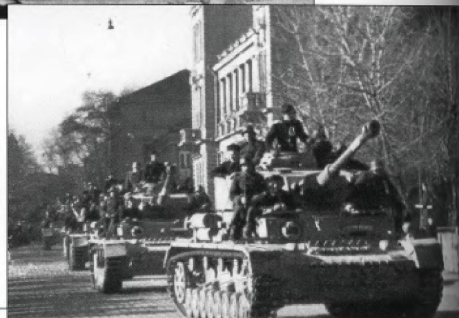
A column of Bulgarian Pz.Kpfw.IV's driving through Sofia in the spring of 1944. From February 1943 to July 1944, the Bulgarian Army received 91 Pz.Kpfw.IV Ausf.G and H from Germany. The lead vehicle is an early Ausf.H fitted with 30mm Zusatzpanzer on the front of the hull and superstructure. In addition to the turret Schürzen, they have been equipped with an engine air filter system called Filzbalgfilter consisting of two cylinders mounted on the right fender. This feature was dropped from production in February 1944.
