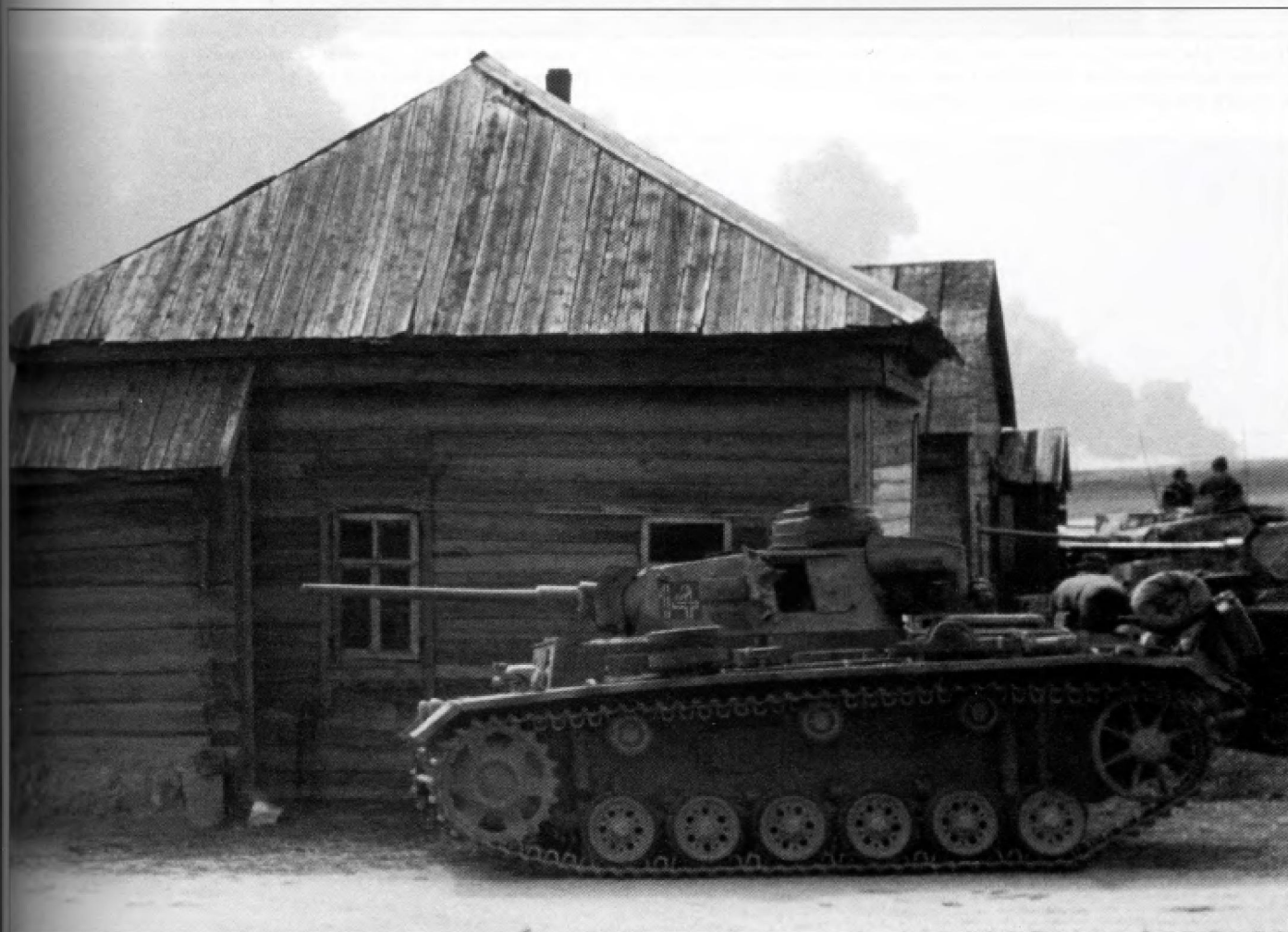
This Pz.Kpfw.III Ausf.J or L appears to be a bit nose heavy, perhaps indicating that one or more of the front torsion bars have been damaged. Judging by the contrast around the white outline tactical number '14' painted on the side of the turret, the vehicle has been painted in a lighter camouflage color over the Dunkelgrau RAL 7021 base coat.
