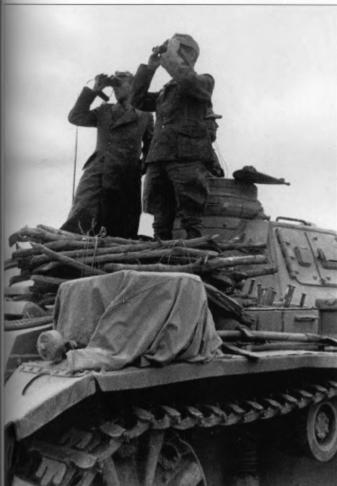
The antenna mounted on the left side and straight back on the turret provide the only evidence that this is a Pz.Bef.Wg.III Ausf.H. A new cast drive sprocket was introduced on the Pz.Kpfw.III Ausf.H however, the early eight hole drive sprocket with a spacer ring to accommodate the new 40cm tracks continued to be used on Pz.Bef.Wg.III.
