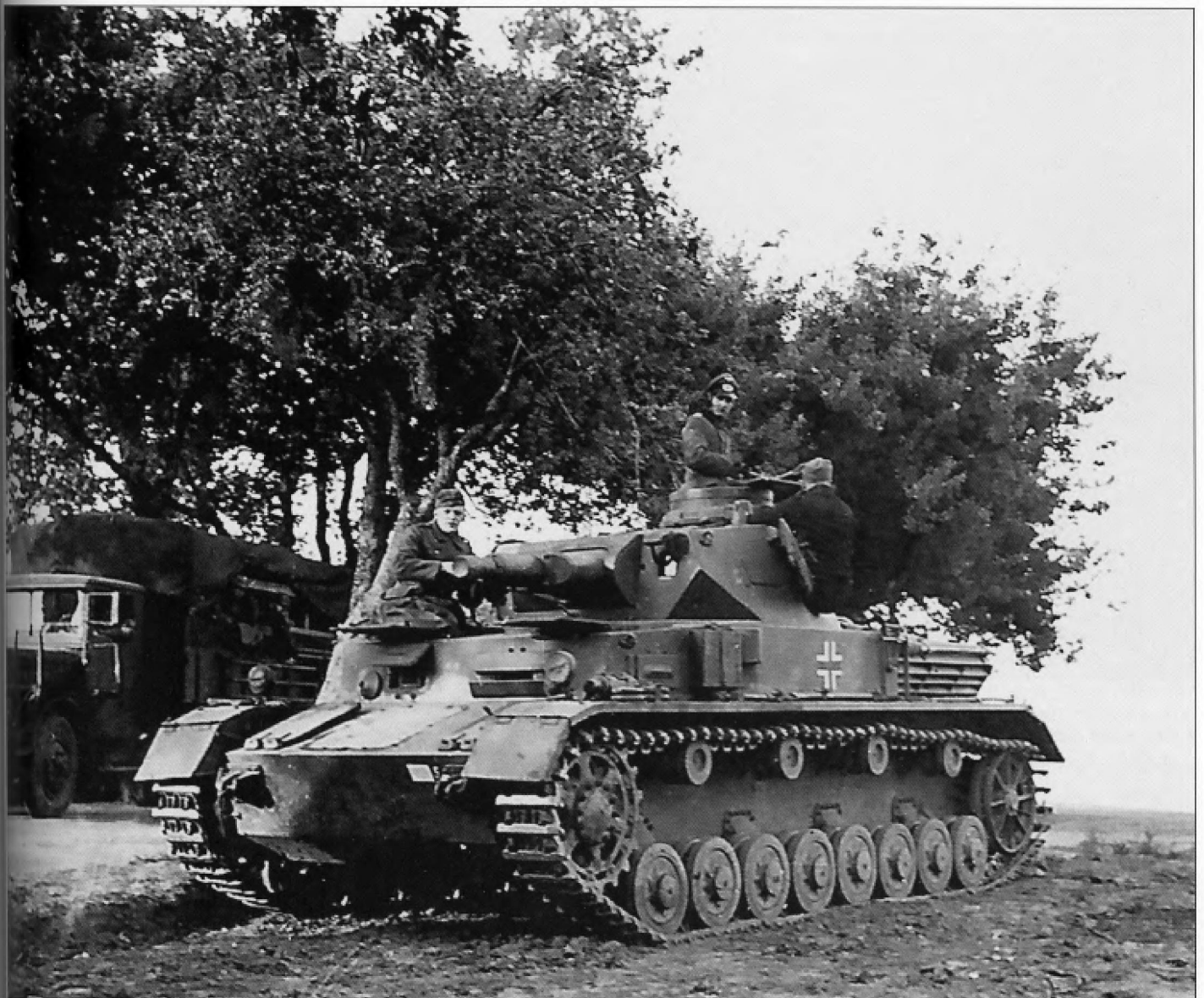
One of the distinguishing features of the Pz.Kpfw.IV Ausf.B and C was the visor and pistol port located in front of the radio operator's position. Another was the steep slope on the engine ventilation grilles which had three horizontal dividers instead of one as seen on the Ausf.D to J. Note the white rhomboid with the number '5' painted on the front plate near the left towing pintle. The tactical emblem for 2.Panzer-Division, two yellow dots, can be seen painted on the front plate between the driver's and radio operator's visors.
