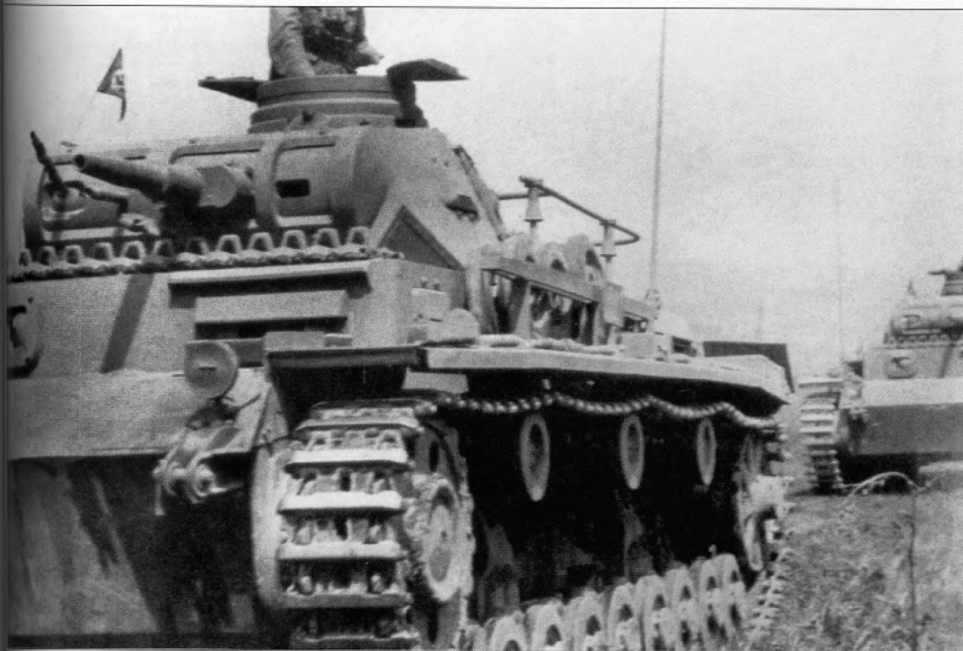
One of the rare Pz.Bef.Wg.III Ausf.D1 seen in France in 1940. It was based on the design of the Pz.Kpfw.III Ausf.D but had additional vision ports and pistol ports in the sides of the hull and was fitted with the driver's visor and hull MG ball mount that was used on the Pz.Kpfw.III Ausf.E. A dummy 3.7cm gun was mounted on the turret which was bolted in place and a large frame antenna was mounted on the engine deck. There were 30 of these vehicles produced from late 1938 to March 1939 and the surviving units were withdrawn from service in early 1941.
