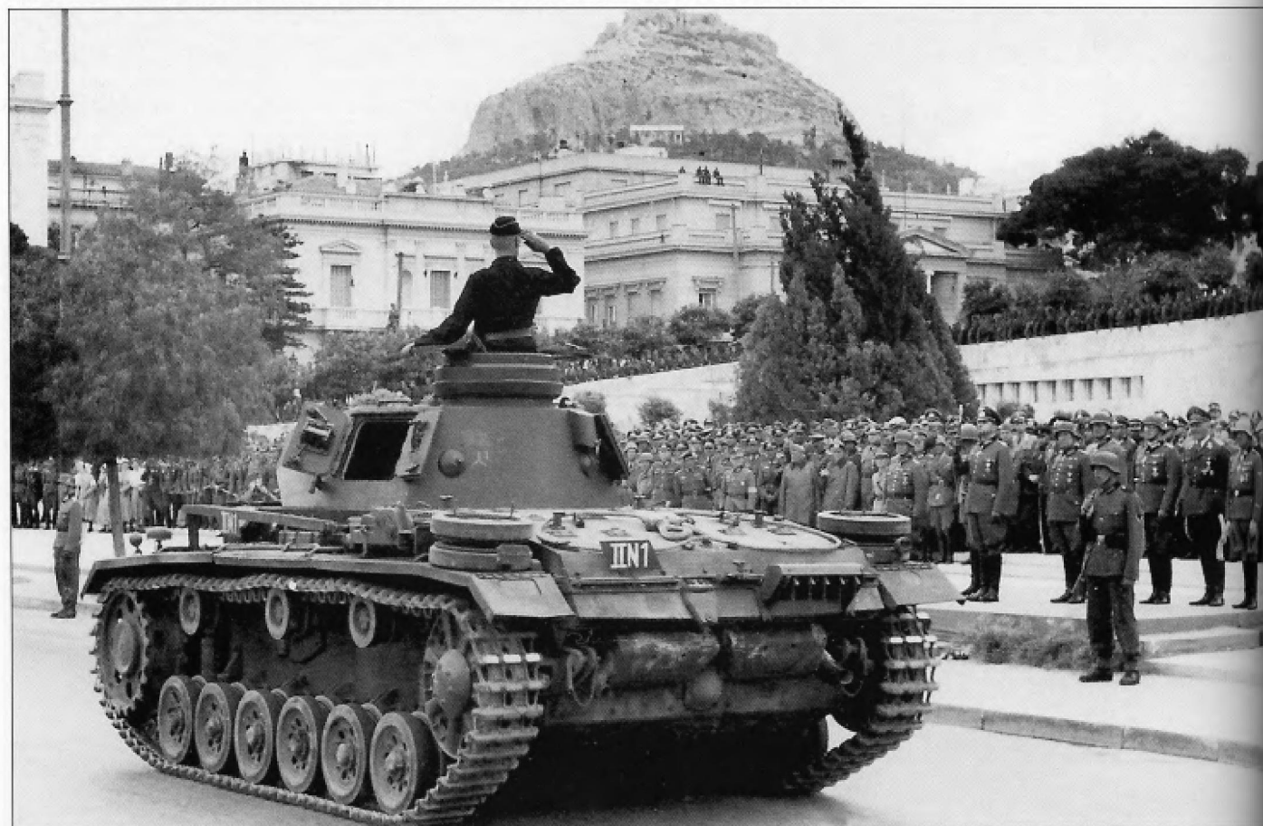
A Pz.Bef.Wg.III Ausf.H from Pz.Rgt.2 of the 2.Panzer-Division drives through the streets of Athens past the Tomb of the Unknown Soldier with Mount Lycabettus rising in the background. It is missing the frame antenna on the engine deck but the mounts for it can still be seen as well as the small armored cover of the antenna wire on the back of the turret. The tactical emblem for 2.Panzer-Division, an inverted 'Y' with a short line beside it can be seen on the back of the turret as well as on the left side of the rear superstructure plate. The tactical number 'II N1' painted on the rhomboid plate indicates that this is the vehicle of the commander of the Nachrichten-Abteilung of the second battalion.
