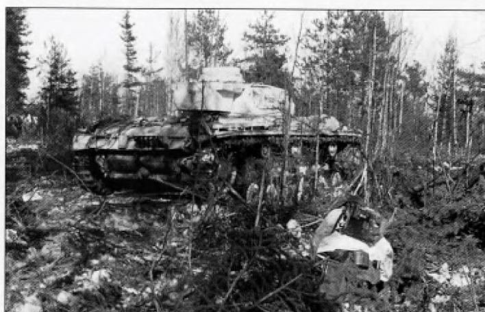
A winter whitewashed Pz.Kpfw.III Ausf.G pushes through a heavily forested area in northern Russia. Unusually, it has been fitted with a turret stowage bin from a Pz.Kpfw.IV.
