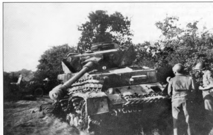
Another Pz.Kpfw.IV Ausf.H from the same unit displaying a complete set of early hull Schürzen modified to fit the new rail system.
