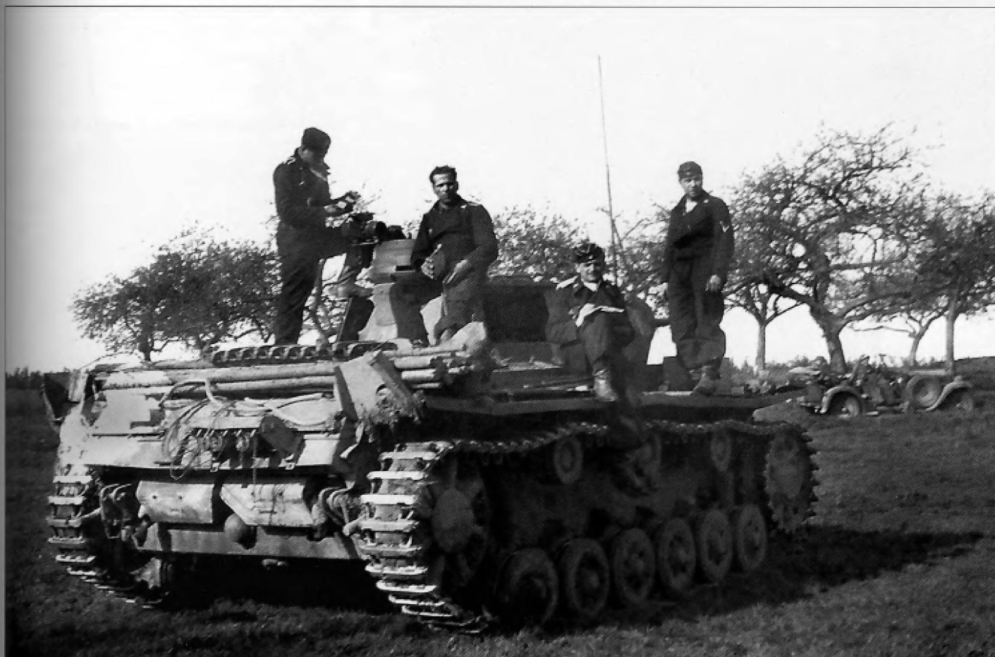
A Pz.Kpfw.III Ausf.E or F sits in a field while its crew relaxes from the rigors of battle. They have cut a bundle of small trees to act as fascines and stored them across the back of the engine deck to be readily available if needed. A smoke candle rack is mounted on the rear of the hull and was operated from inside the vehicle by a mechanism connected to the rack by means of a steel cable. Only two of the five smoke candles remain.
