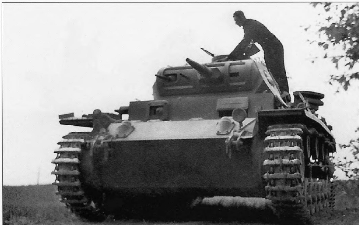
This Pz.Bef.Wg.III Ausf.E is unusual in that it has a hinged flap covering the opening for the driver's visor instead of the normal Fahrersehklappe 30. The main armament was replaced by a dummy gun to provide more space inside the turret and a dummy machine gun and a ball mount for an MG34 were installed in the mantlet. The fixed turret was moved forward on the hull and the turret ring was replaced by an opening that matched the shape of the base of the turret. The antenna mount on the right side of the vehicle was moved forward as well and can be seen here on the left side of the photo. Armored brake cooling vents have also been fitted to glacis. Only 45 of these vehicles were produced from July 1939 to February 1940.
