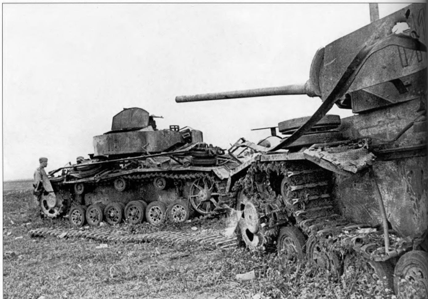
The same two vehicles seen from the opposite side. The one on the left is a Pz.Kpfw.III Ausf.L while the one on the right is an Ausf.M. They are from Pz.Rgt.3 of the 3.SS-Panzer-Grenadier-Division 'Totenkopf' and were knocked out in the Kursk area in July 1943.
