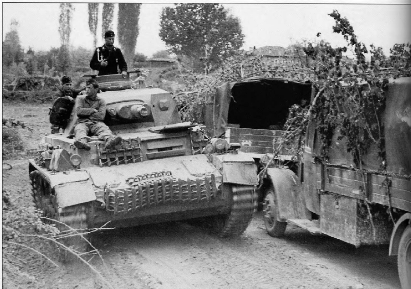
The armored sleeve on the coaxial machine gun provides proof that this is a Pz.Kpfw.IV Ausf.C. The chassis number of the vehicle is painted on the end of the muzzle dust cover, an early common practice also seen on variously on jacks, jack blocks and the hull itself.
