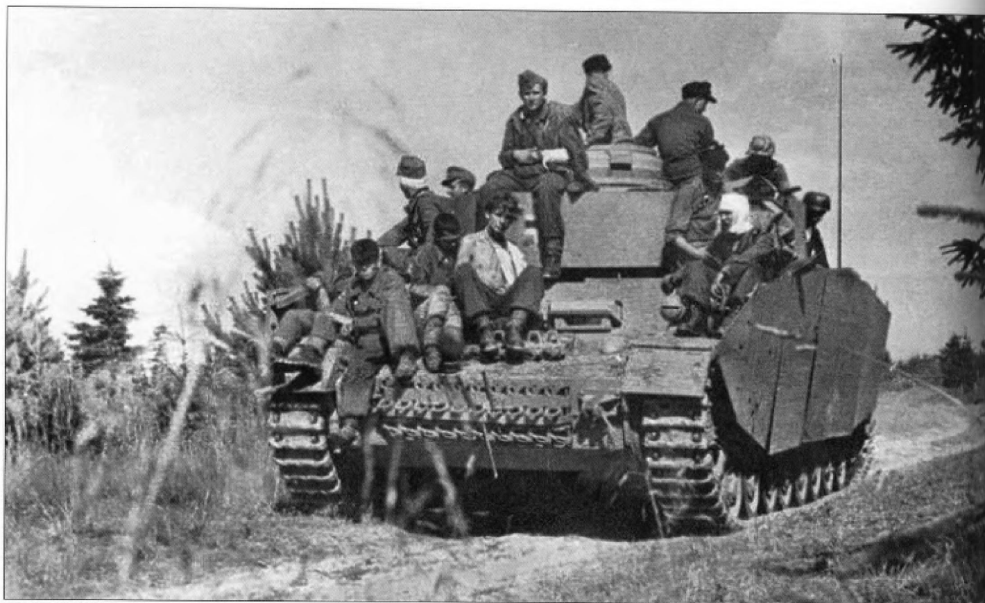
This Pz.Kpfw.IV Ausf.H or J is being used to ferry wounded soldiers to a rear area. It has a coat of Zimmerit and the later style forged hub caps can be seen on the road wheels. The general condition and the fact it still has a full set of hull Schürzen indicates it has not seen much action.
