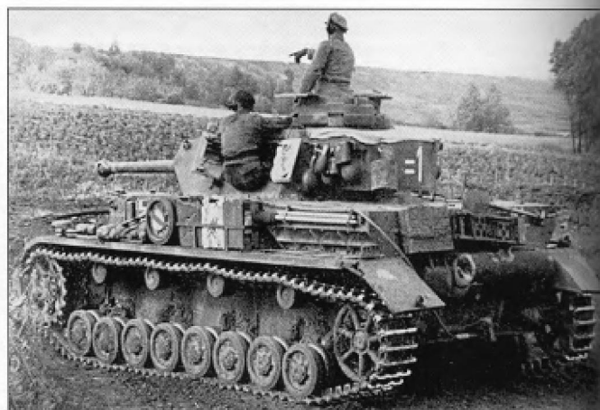
The early Pz.Kpfw.IV Ausf.F2 was fitted with a single baffle round muzzle brake. Approximately 238 were produced from March to July 1942 before the name was changed but it is not known how many were completed with the early muzzle brake. This one is from 2./Pz.Abt. 'Großdeutschland', which was equipped with 12 Pz.Kpfw.IV Ausf.F2(G) in July 1942. At this time, the Abteilung employed a unique method of marking their vehicles using either one, two or three horizontal lines representing the company followed by a single digit. The divisional emblem, a white 'stahlhelm' can be seen painted on the left hinged mudguard.
