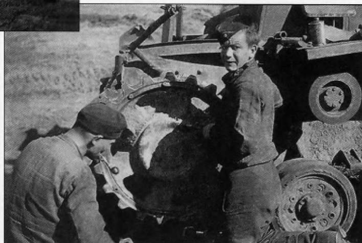
Two crew members of this Pz.Kpfw.III Ausf.J work to replace a damaged drive sprocket ring. The hull side extension that was drilled out for towing can just be seen over the head of the crewman on the left as well as the redesigned armored brake cooling vent that was introduced on the Ausf.J. The skewed angle on the front fender support brace suggests that the damage may have been caused by a mine although the first road wheel and track lying below the sprocket do not appear to be damaged.
