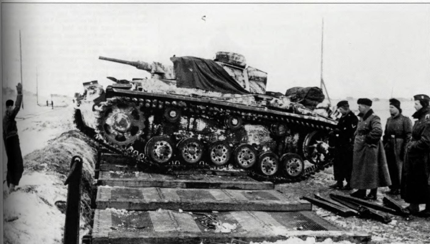
The Pz.Kpfw.III Ausf.J featured short extensions of the hull side plates that were drilled for towing in place of the earlier cast tow pintles. A new cast drive sprocket was introduced on the Ausf.H and continued to be used until the end of the war. The 5cm KwK L/42 gun continued to be used until appearance of the long barrel 5cm KwK L/60 gun in early 1942. This vehicle has obviously seen some action as one segment of the cupola visors has been shot away.
