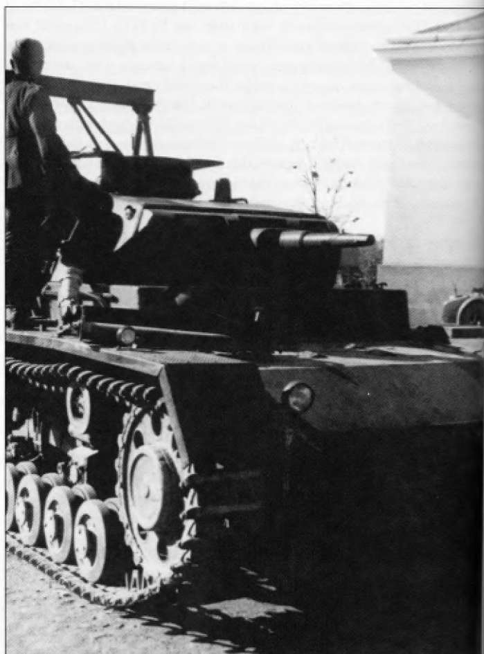
The Pz.Kpfw.III Ausf.C utilized an eight wheel suspension system with leaf springs similar to the Ausf.B and Ausf.D. This vehicle can be identified as an Ausf.C from the type of drive sprocket and the location of the front shock absorber which can be seen just below and behind the forward return roller. It was also lightly armored but did see combat in Poland. A total of 15 vehicles were produced in 1937 and early 1938 and were withdrawn from service in 1940.
