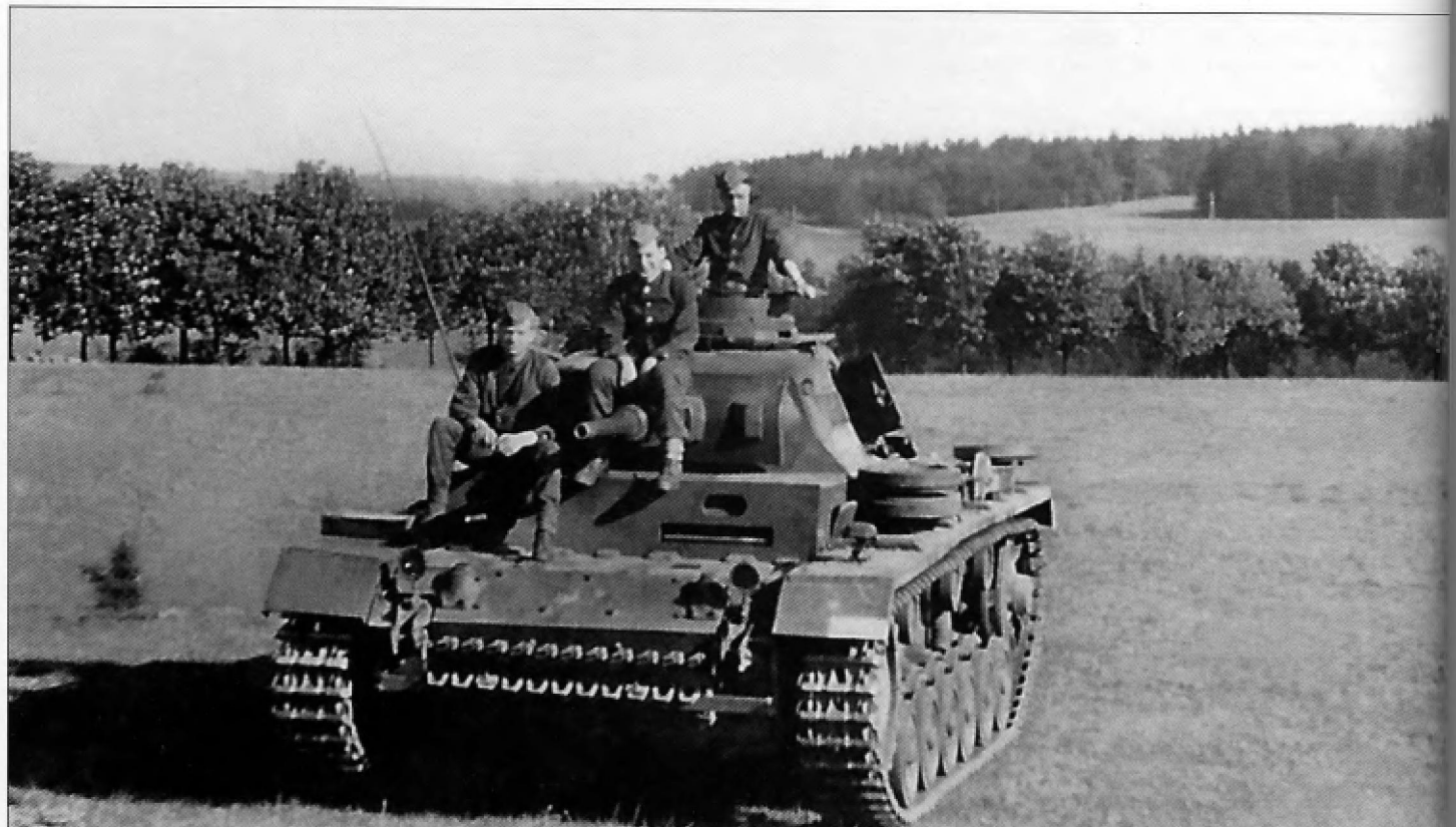
Another modified Pz.Kpfw.III Ausf.F. The additional 30mm armor plates bolted to the glacis are evident as are the cutouts in the 30mm plate for the driver's visor and periscope. The Notek light has been relocated to the left fender and two spare road wheels mounted. It is also fitted with the early cupola.
