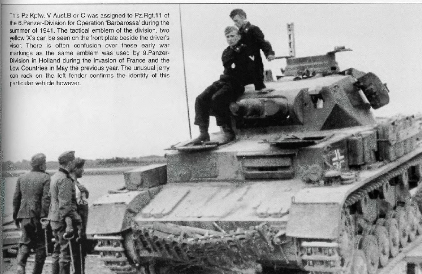
The wooden antenna trough is missing off this battle scarred Pz.Kpfw.IV Ausf.B or C along with most of the tools normally carried and the hinged mudguards. The tactical number '813' is painted in white on a black metal rhomboid plate following standard early practice. This would have been carried on both sides and the rear of the vehicle. Note how the dust has completely covered lower parts of the hull and running gear.
