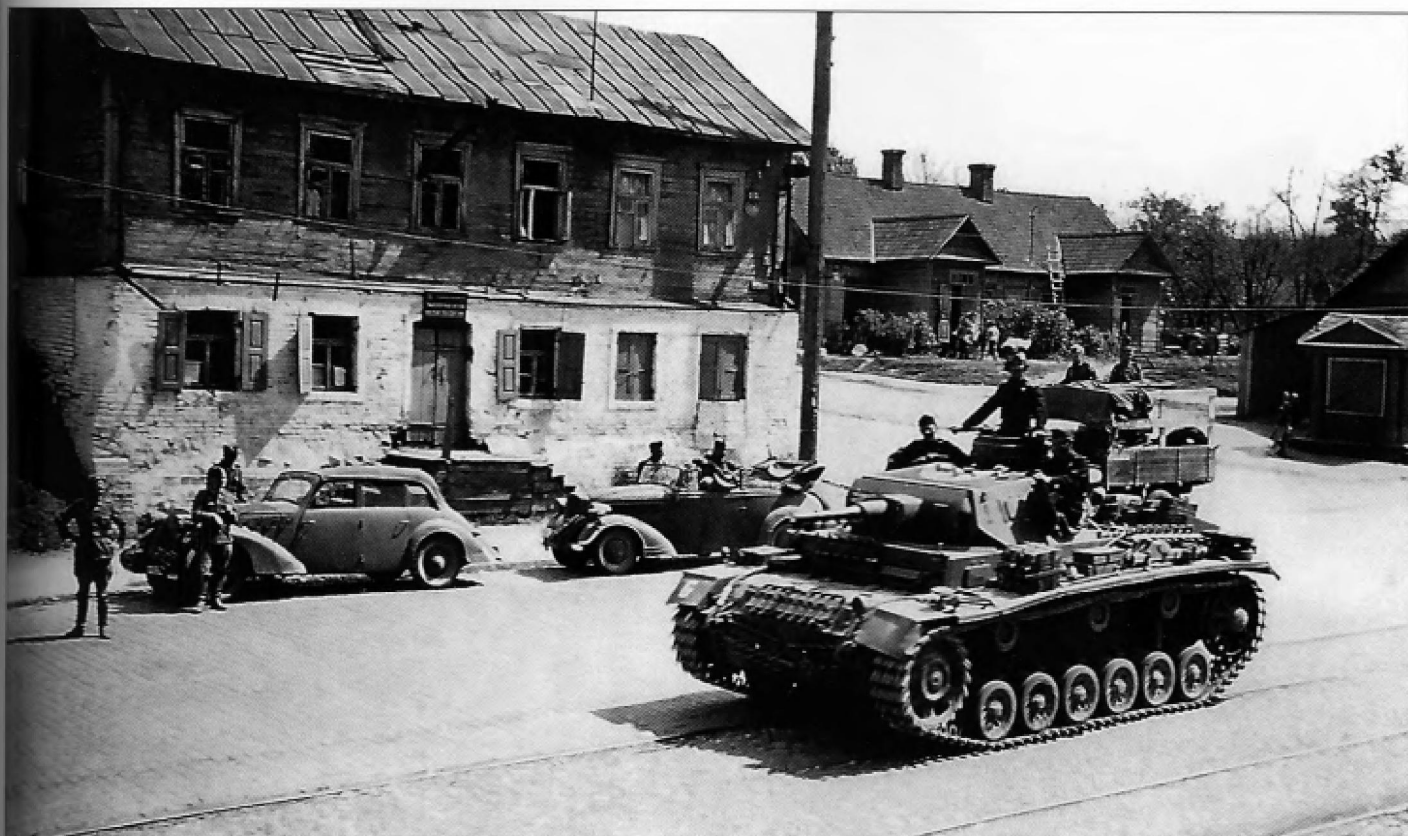
A Pz.Kpfw.III Ausf.J fitted with the 5cm KwK L/42 gun rolls through a Russian town during the summer of 1942. There were 1,549 Pz.Kpfw.III with the short barrel 5cm gun produced from March 1941 to July 1942.
