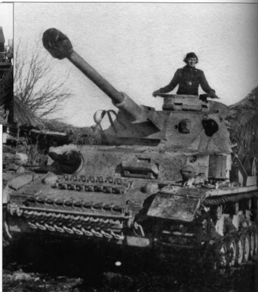
The 30mm Zusatzpanzer and antenna deflector can be clearly seen on this new Pz.Kpfw.IV Ausf.G seen in Russia in the summer of 1942. Unusually, a shipping stencil can be seen painted on the lower front side of the turret. The light color suggests that it is also painted in a tropical scheme. The final drives on the Ausf.A to Ausf.G were protected with curved armor plates bolted to the housing which can be clearly seen in this photo. Reinforced final drive housings were introduced on the Ausf.H which eliminated the curved plates.
