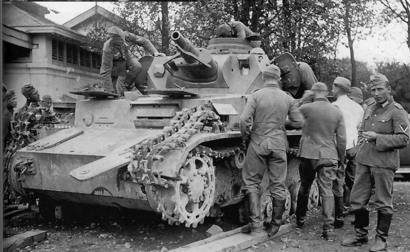
A damaged Pz.Kpfw.IV Ausf.C is inspected by curious German soldiers. The armored sleeve is clearly visible in this photo as are the radio operator's visor and pistol port and the antenna deflector mounted on the main gun. The very light color of the vehicle appears due to remains of a well applied winter whitewash paint.
