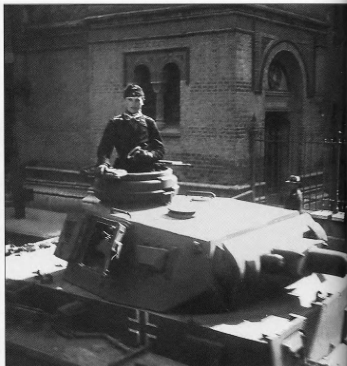
This view of a Pz.Kpfw.III Ausf.H provides a look at how the additional 30mm face hardened armor plate on the front of the superstructure was higher than the roof above the driver and radio operator. The new cupola can also be seen to good effect as well.
