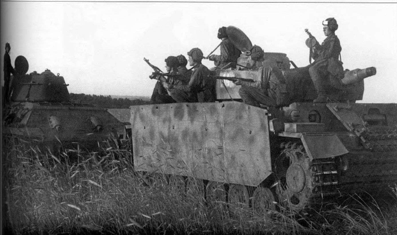
This captured late production Pz.Kpfw.III Ausf.N was built on the chassis of a Pz.Kpfw.III Ausf.M and is fitted with turret and hull skirt armor and the late one-piece cupola hatch. It is being towed by the T-34 to the left and the Soviet troops are simply striking a pose for the cameraman.
