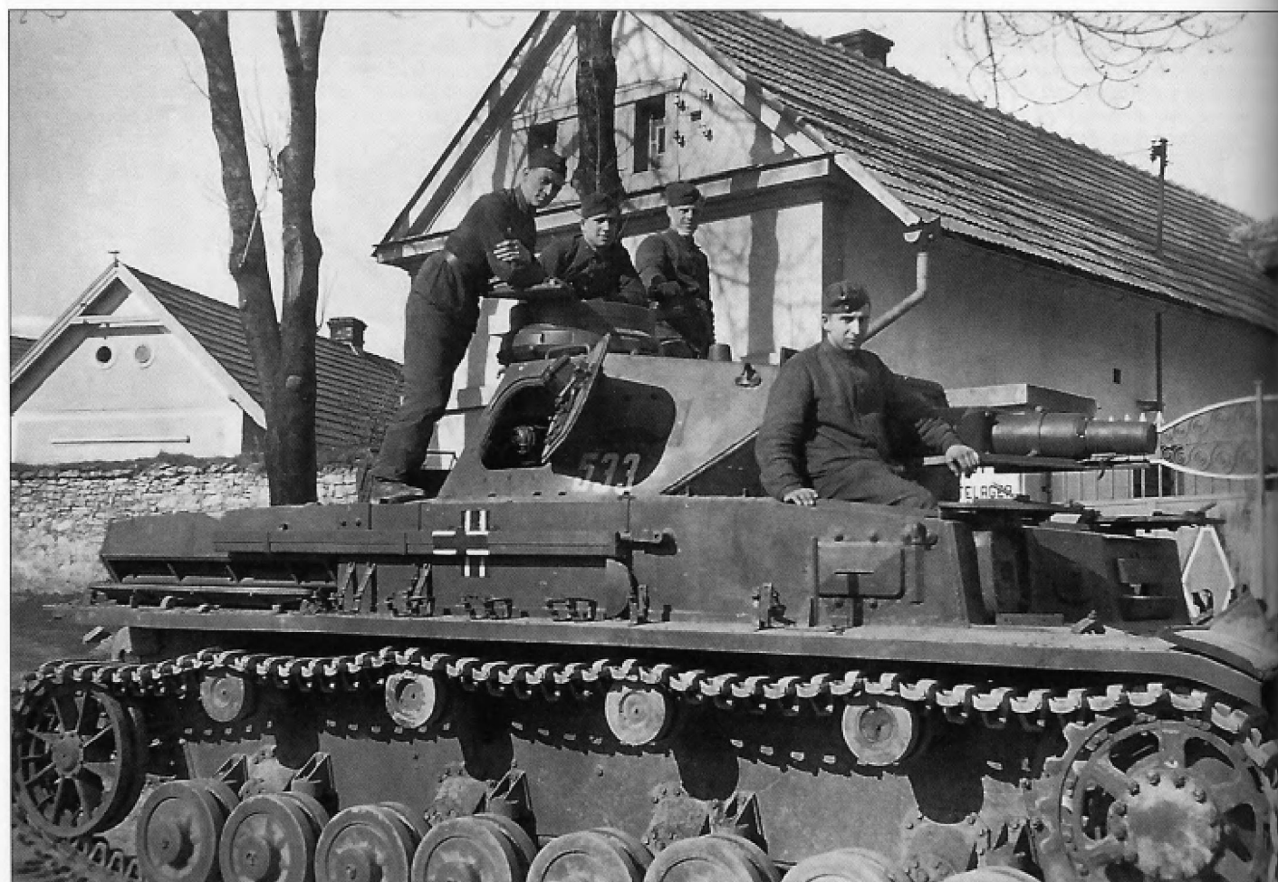
Another Pz.Kpfw.IV converted to a Tauchpanzer from Pz.Rgt.18 of the 18.Panzer-Division. Similarly to the Pz.Kpfw.III, a bolt flange was added around the front of the turret and hull MG mount for attaching water tight covers for deep wading. The tactical emblem, a yellow 'Y' with three horizontal lines through the tail, can be faintly seen in front of the tactical number '533'.
