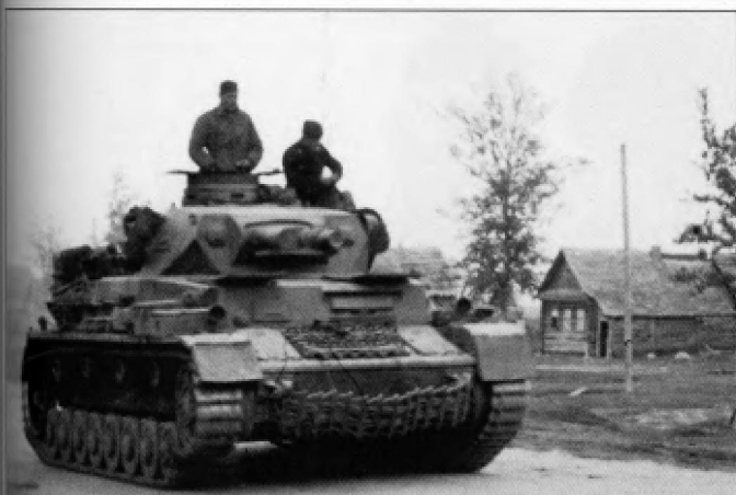
This Pz.Kpfw.IV Ausf.C has been fitted with an additional 30mm armored plate on the front of the lower hull.
