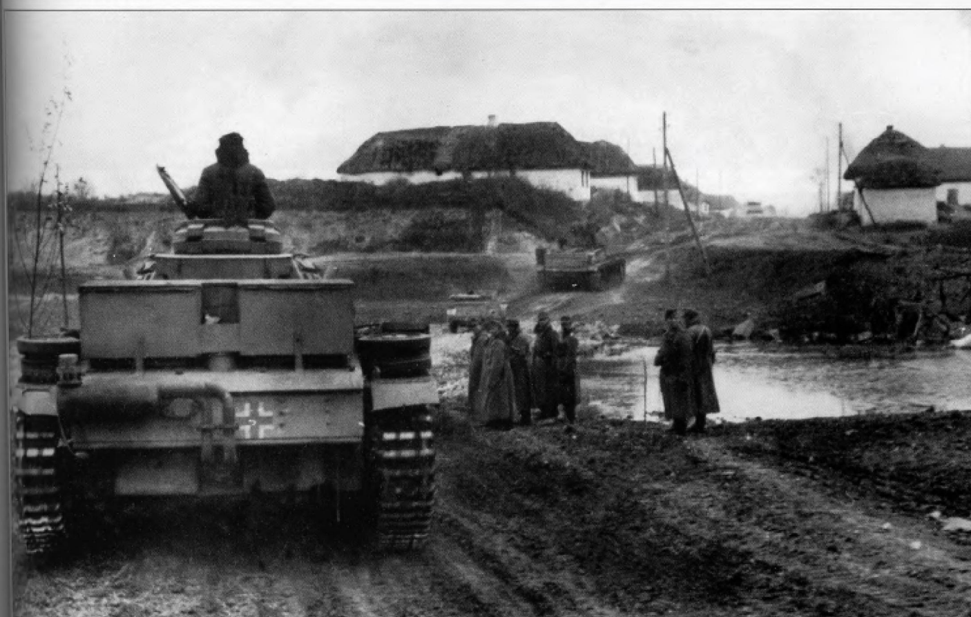
The Pz.Bef.Wg.III Ausf.K utilized a modified Pz.Kpfw.IV Ausf.F or Ausf.G turret mounted on a Pz.Kpfw.III Ausf.M chassis. The main armament was the 5cm KwK L/60 gun mounted on a narrow Pz.Kpfw.III mantlet leaving space for a pivoting visor, similar to the driver's visor, on the right side of the gun. A star antenna mounted on the engine deck replaced the large frame antenna. This vehicle is the personal mount of Oberst Graf von Strachwitz, commander of Pz.Pgt. 'Großdeutschland' and was photographed near Kharkov in March 1943. Other photographs of this vehicle show that it still retains the side escape hatches that were dropped during production of the early Pz.Kpfw.III Ausf.L.
