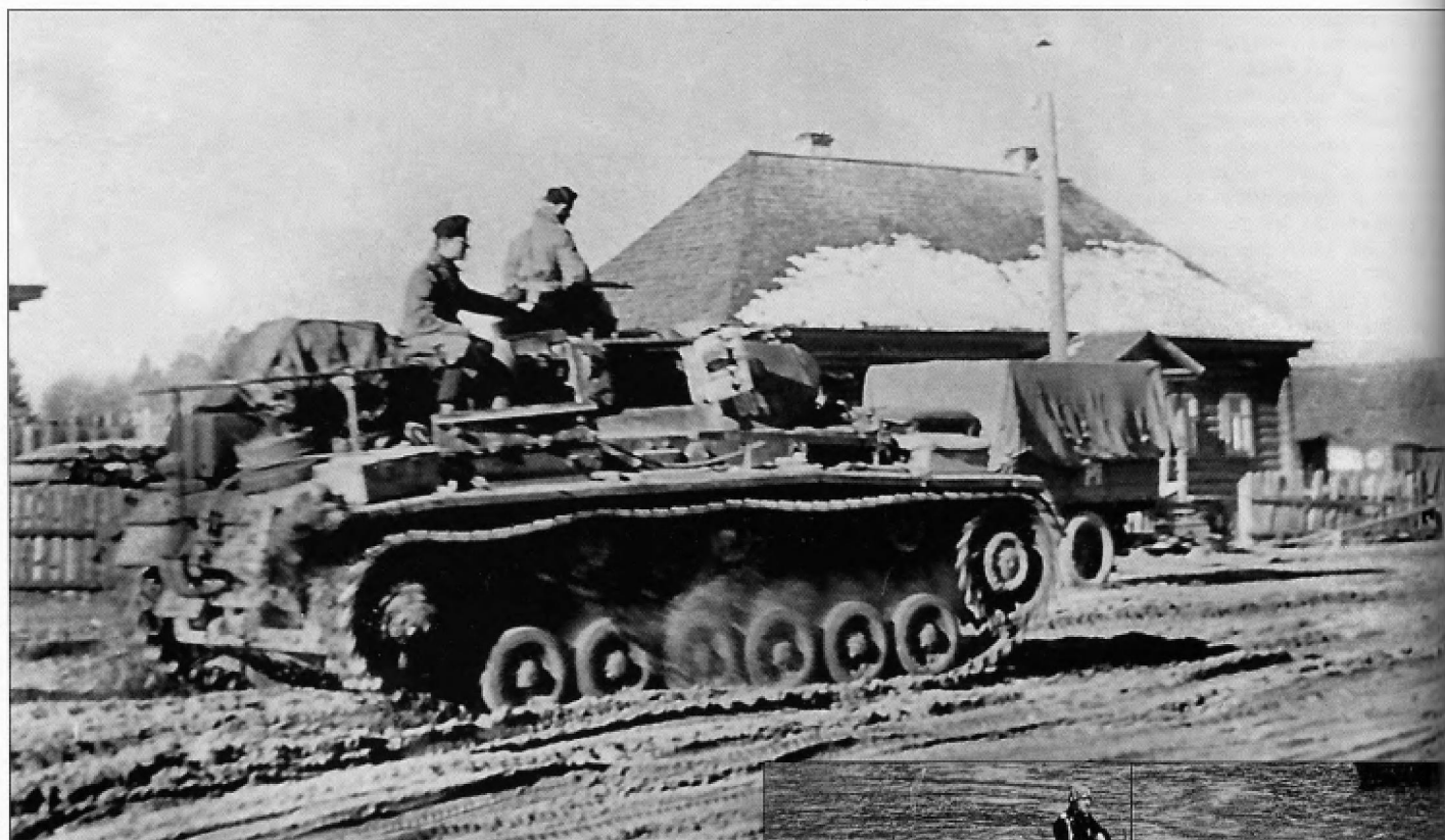
Another Pz.Bef.Wg.III Ausf.H that has been converted to a Tauchpanzer as can be seen by the curved exhaust pipes projecting from under the rear plate and the raised watertight door on the air intake on the side of the engine deck. Although the engine deck has been piled high with stowage, the outline of the frame antenna can clearly be seen. It is likely that this vehicle was also assigned to 18.Panzer-Division. (Photo courtesy of John Prigent)
