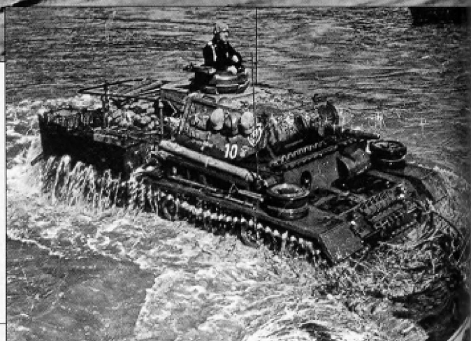
Another Pz.Bef.Wg.III Ausf.H that has been converted to a Tauchpanzer as can be seen by the curved exhaust pipes projecting from under the rear plate and the raised watertight door on the air intake on the side of the engine deck. Although the engine deck has been piled high with stowage, the outline of the frame antenna can clearly be seen. It is likely that this vehicle was also assigned to 18.Panzer-Division. (Photo courtesy of John Prigent)
