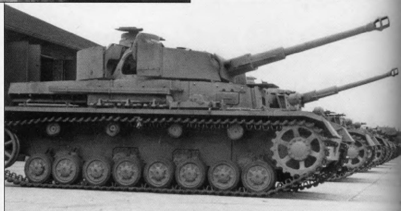
All Pz.Kpfw.IV Ausf.D returned for refurbishing after July 1942, were upgraded with the 7.5cm KwK L/48 gun, 40cm tracks, 90mm wide road wheels and drive sprockets and idler wheels from Pz.Kpfw.IV Ausf.G production. The turret Schürzen were added sometime after they were introduced into production in May 1943. Photos of these vehicles used in combat are rare with at least one being knocked out in Italy.
