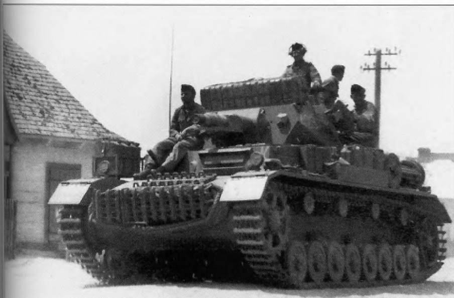
This Pz.Kpfw.IV Ausf.D from one of the Panzer-Division in Gruppe von Kleist is notable for its left front drive sprocket which was from a Pz.Kpfw.IV Ausf.E. Special racks on the fenders and turret roof carry no less than 14 jerry cans of fuel for the attack on the Soviet Union on June 22, 1941. The tactical number '423' can be seen painted in white on the side of the turret.
