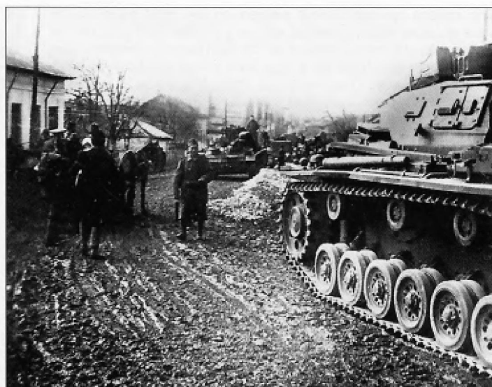
The antenna mounted on the left side and straight back on the turret provide the only evidence that this is a Pz.Bef.Wg.III Ausf.H. A new cast drive sprocket was introduced on the Pz.Kpfw.III Ausf.H however, the early eight hole drive sprocket with a spacer ring to accommodate the new 40cm tracks continued to be used on Pz.Bef.Wg.III.
