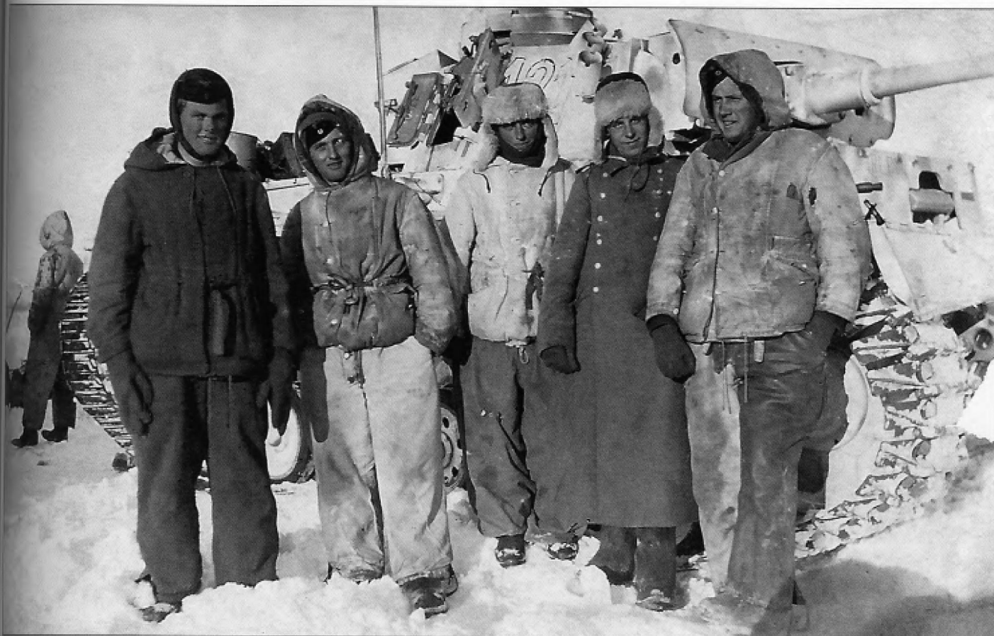
A smoke discharger rack was installed on each side of the turret beginning with the Pz.Kpfw.III Ausf.M. This vehicle has also been fitted with special wide 'Winterkette' winter tracks that provided increased traction in deep snow and were issued to Panzer III and StuG.III units on the Eastern Front only. By this time a variety of warm winter clothing was available to the Panzer crewmen.
