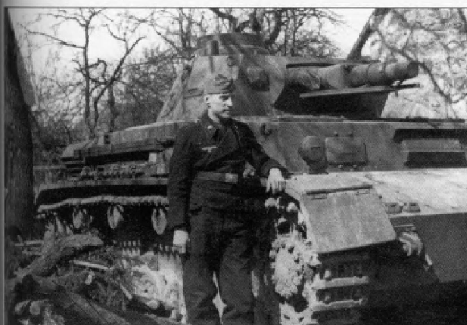
This Pz.Kpfw.IV Ausf.C has been fitted with an additional 30mm armored plate on the front of the lower hull.
