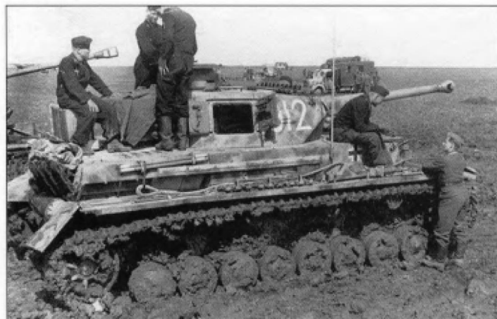
An armored brake cooling vent was added to the brake access hatches on the glacis. The new drive sprocket and idler design along with the two-piece turret side hatches can be seen in this photo. Other improvements include a new shorter muffler, modifying the turret traverse motor muffler and redesigning and moving the armored smoke candle rack to the left side of the rear plate. There were 462 Pz.Kpfw.IV Ausf.F produced from April 1941 to March 1942.
