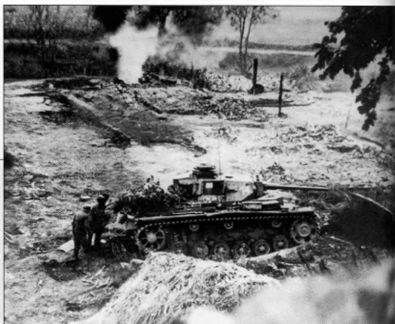
A Pz.Kpfw.III Ausf.J or L sits amid the burning ruins of a Russian village. The turret side visor was still being installed on early production Ausf.L along with hull side escape hatches, making an exact identification impossible. The tactical number '14' can be seen painted in white on the side of the turret.
