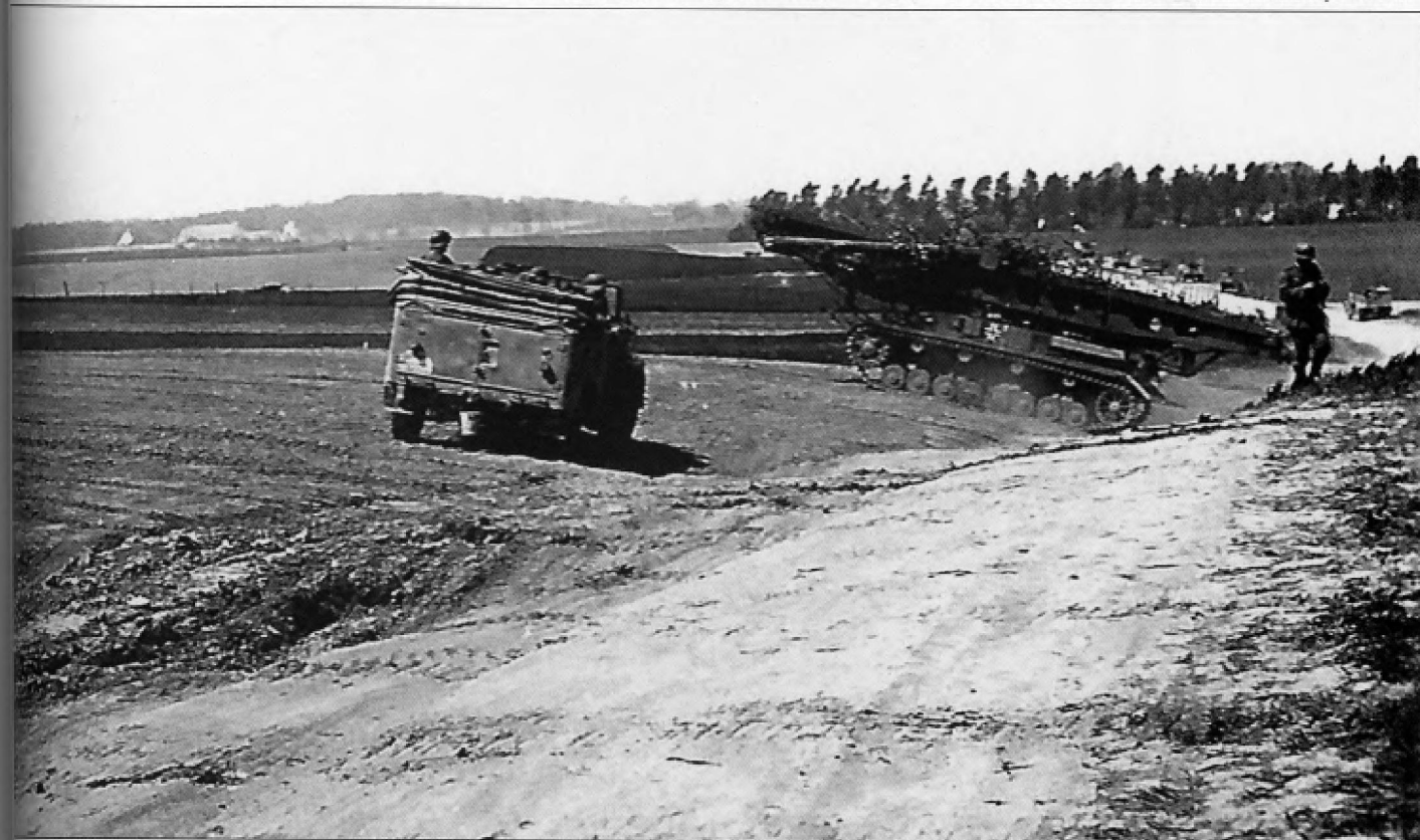
Twenty Pz.Kpfw.IV Ausf.C and D were converted to Brückenleger IV or bridge layer tanks which mainly saw service in the Panzer Division in 1940. Two bridge designs were used, one by Krupp as seen here and one by Magirus. Further production was cancelled after the battle of France and most were re-converted back into gun tanks.
