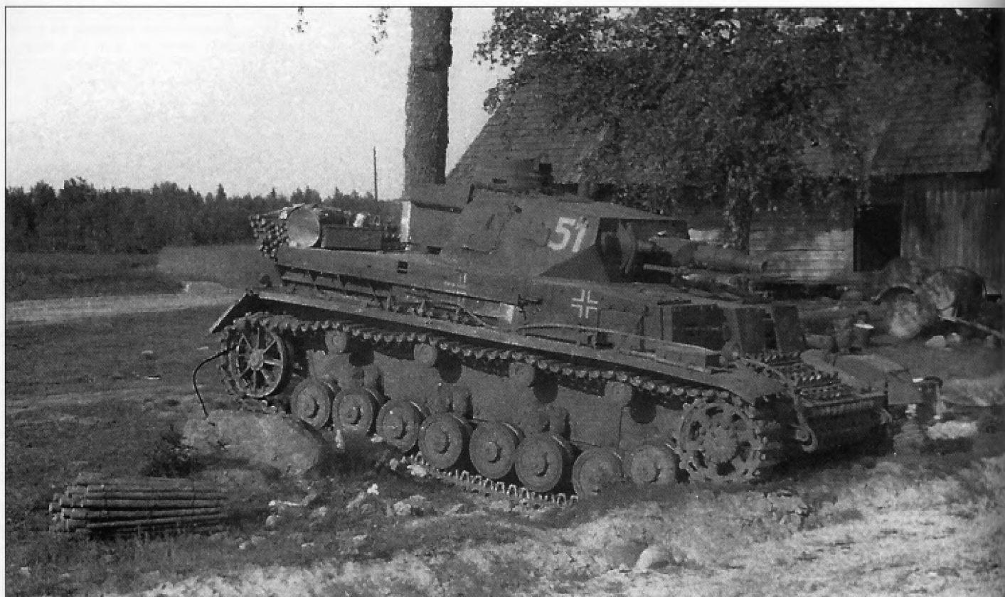
This Pz.Kpfw.IV Ausf.D has been fitted with additional 30mm armor plates to the front and sides of the superstructure and sides of the hull that were introduced in July 1940. The tactical number '51' is unusual in that Pz.Kpfw.IV's were normally assigned to either the 3. or 6.Kompanie in Abteilung with three companies or the 4. or 8.Kompanie in Abteilung with four companies.
