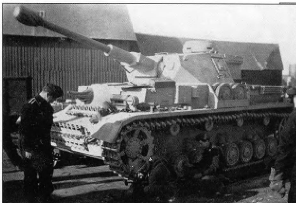
A new Pz.Kpfw.IV Ausf.G in a tropical paint scheme, being secured for rail transport to the front. The spare road wheel storage bin on the left fender and spare track brackets on the glacis can be seen in this photo. The gun barrel is also painted with dark grey heat resistant primer and an antenna deflector has been added on the right side of the mantlet. Starting in May 1942, some Pz.Kpfw.IV Ausf.F2 and G had 30mm armor plates, called Zusatzpanzer, welded to the front of the superstructure and hull.
