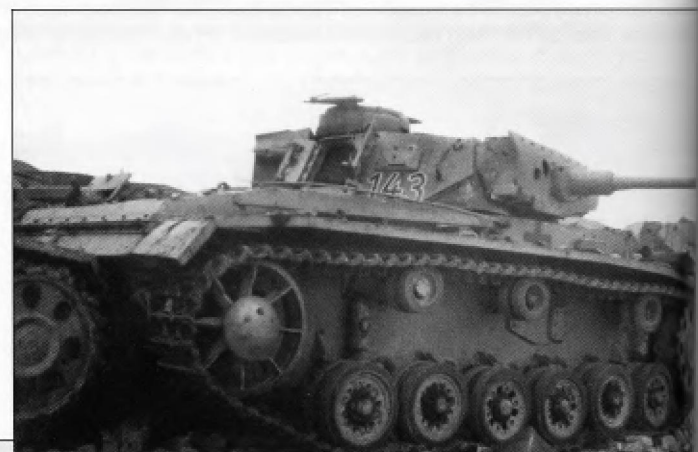
Judging by the way these Pz.Kpfw.III's are jammed together, they are probably in a Soviet vehicle dump. This Pz.Kpfw.III Ausf.H still has the early eight-hole drive sprocket with spacer rings for the 40cm tracks but has been fitted with the new welded idler and improved shock absorbers. In addition, it has the 20mm spaced armor plates that were introduced during production of the Pz.Kpfw.III Ausf.L and been fitted to some Ausf.H and J. It appears that this vehicle has been painted in overall dark yellow and has an unusual black Balkenkreuz without white outline.
