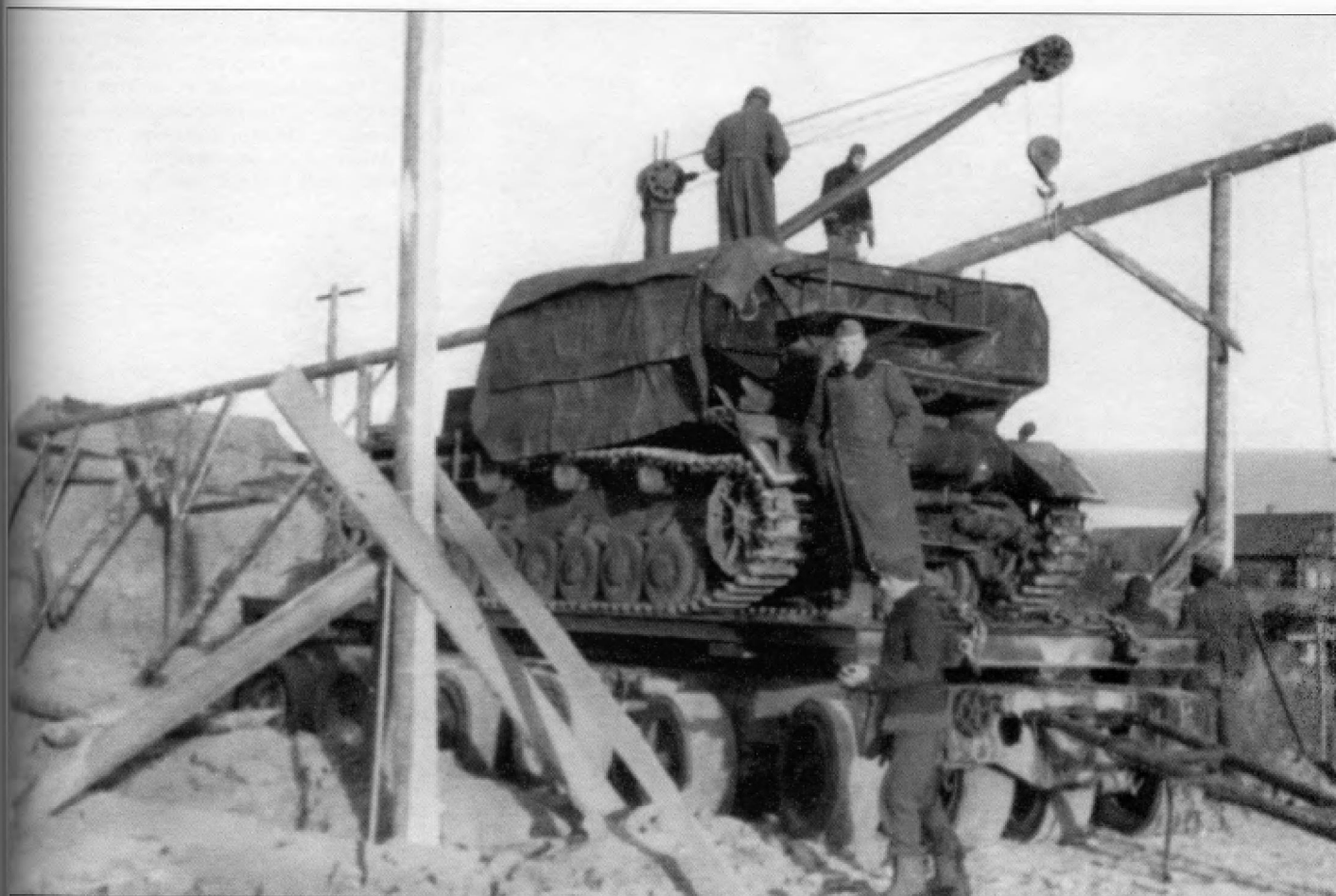
This ungainly looking vehicle is a Munitionsschlepper für Karlgerät, or munitions carrier for the 60cm self-propelled heavy siege mortar known as the 'Karl'. Initially built on the chassis of the Pz.Kpfw.IV Ausf.D like this one, some were later constructed on Pz.Kpfw.IV Ausf.F chassis as well as some on rebuilt Pz.Kpfw.IV chassis. It carried four rounds of 60cm ammunition in the box-like superstructure and was fitted with a small crane to handle the heavy rounds.
