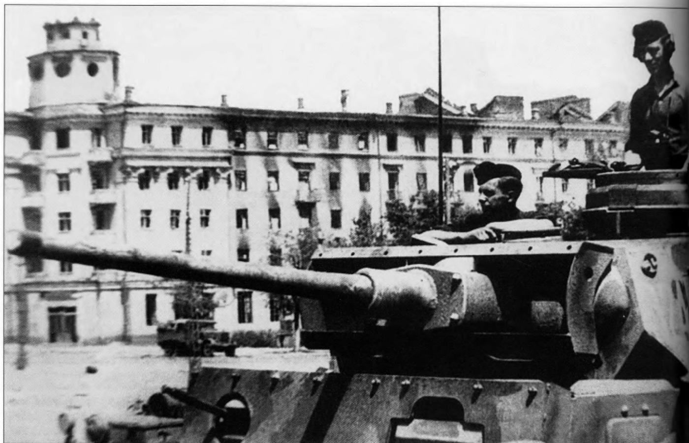
This Pz.Kpfw.III Ausf.J or L was photographed in the Russian city of Voronezh in the summer of 1942. It appears to have had a two color camouflage paint scheme applied over the Dunkelgrau base. The tactical number '324' is painted in white on the side of the turret and, like most of the early production Ausf.J, is missing the 30mm armor plate on the mantlet.
