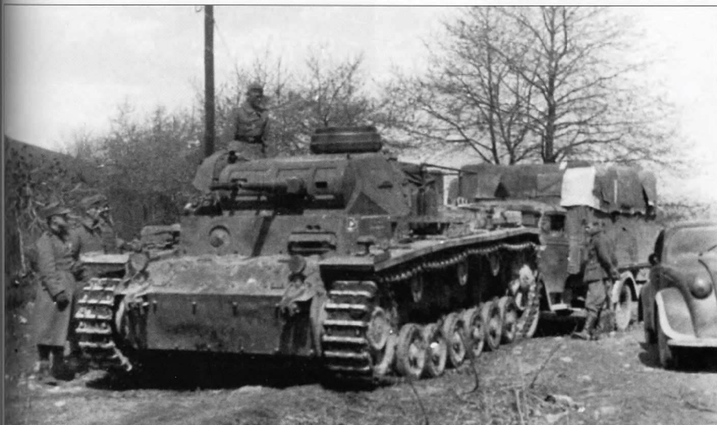
An early Pz.Bef.Wg.III Ausf.H fitted with the early 3.7cm dummy gun. A pistol port replaced the ball machine gun mount in the front plate. The lifting hooks for the turret were mounted on the roof instead of the sides and rear as on a standard Panzer III. The tactical sign for a Nachrichten-Abteilung is painted in white outline on the top left corner of the front plate with a solid white tactical sign for a Panzer-Division Stab, a rhomboid with a small flag on top, painted inside of it.
