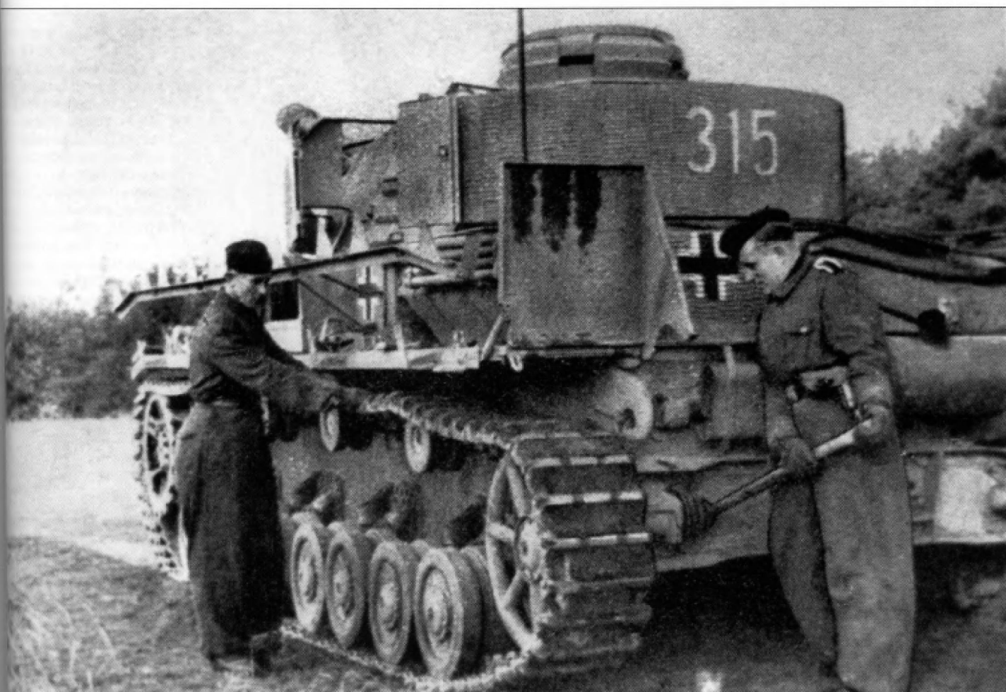
Another example of an early Pz.Kpfw.IV Ausf.H with Zimmerit applied to the turret Schürzen. The later style of hull Schürzen support angle has been fitted to this vehicle which had triangular teeth welded to it and modified hooks mounted to the fenders which engaged brackets welded to the inside face of the plates. The crewman at the back of the tank is using the track wrench to adjust the track tension. The three dark strips on the underside of the hinged mudguard were caused by the track cleats throwing up dirt and sand particles which have removed the paint.
