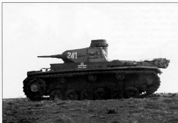
This Pz.Kpfw.III Ausf.E or F also has a bundle of fascines strapped to the engine deck. Note the lack of a raised periscope cover on the turret roof.
