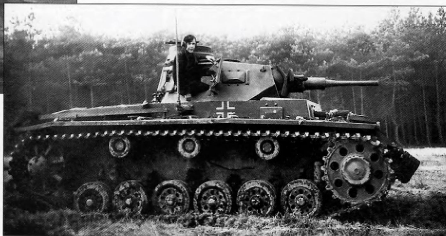
This early Pz.Kpfw.III Ausf.G has had the barrel of its 3.7cm gun shot off during an engagement in Russia. It is still fitted with the early cupola, 75mm wide rubber tired road wheels and 38cm tracks. An improved pivoting driver's visor, the Fahrersehklappe 30 was introduced on the Ausf.G. A white tactical sign for a Panzer-Division is painted on the left mudguard followed by the number '3' indicating the company to which the vehicle was assigned.
