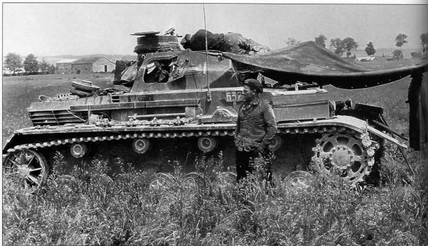
This photo of a Pz.Kpfw.IV Ausf.B or C provides a good view of the early engine ventilation grilles. Judging from the fixed tarp and exposed position, combat is not imminent. The maximum armor thickness on the Pz.Kpfw.IV Ausf.B and C was 30mm on the front of the turret, superstructure and hull and 15mm on the sides and rear.
