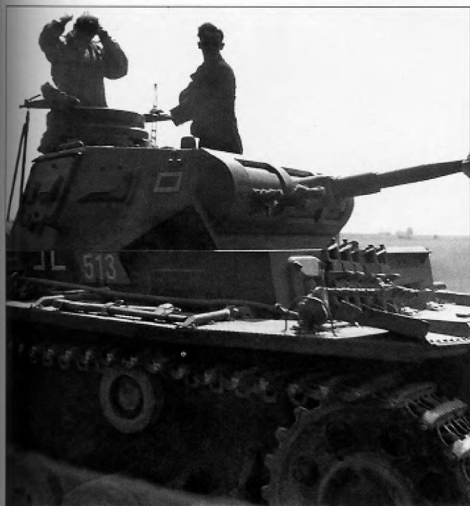
A Pz.Kpfw.III Ausf.E or F from Pz.Rgt.3 of 2.Panzer-Division during the advance through the Balkans in April 1941. Note the radio operator's visor on the right side of the hull and the raised periscope cover on the turret roof. During this time, this division employed a system of marking their vehicle with small geometric shapes on the side of the turret, the meaning of which is not clear. The tactical number '513' is painted on a small rhomboid plate which would also have been seen on the left fender and rear hull.
