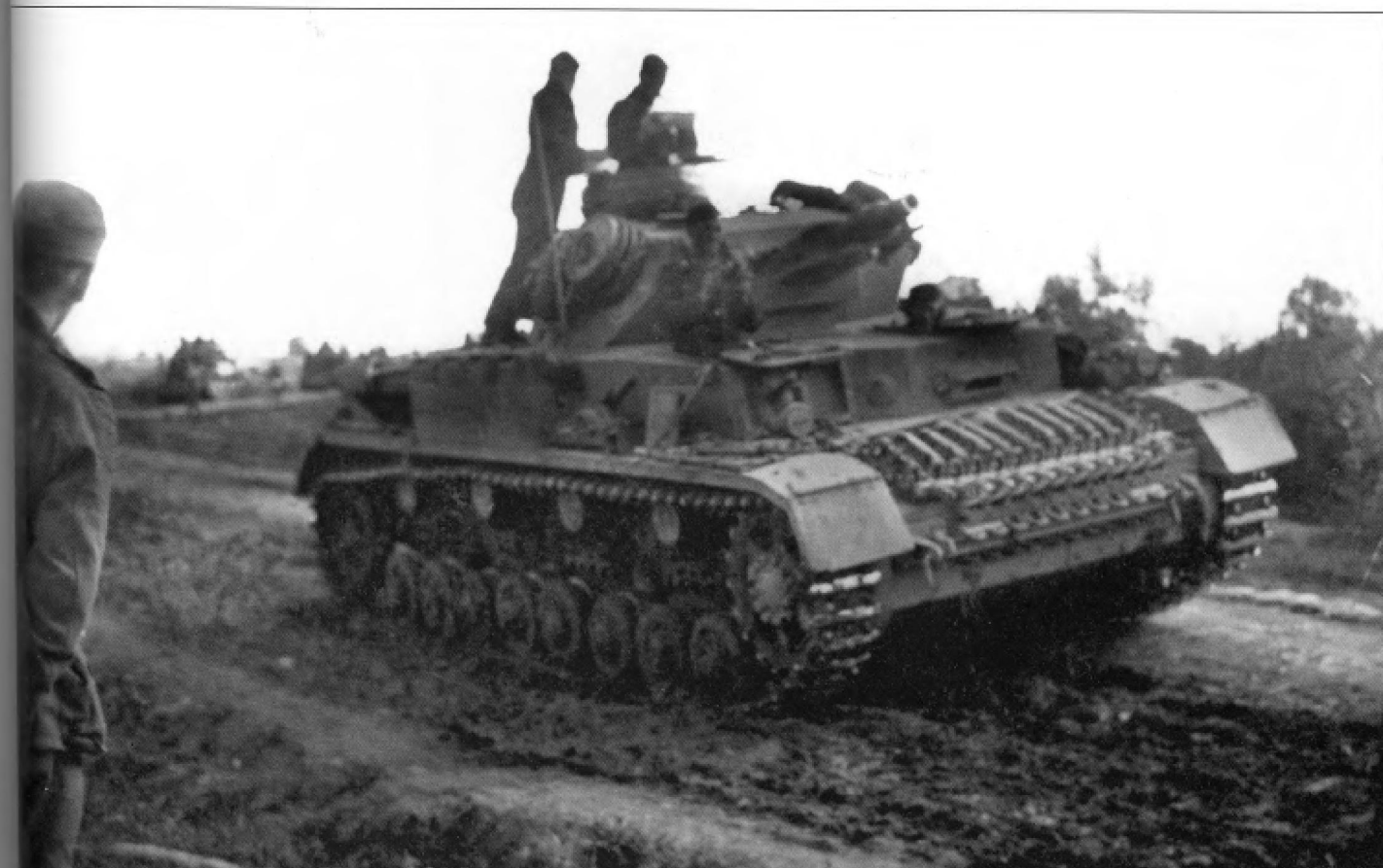
Another Pz.Kpfw.IV Ausf.E converted to a Tauchpanzer. This is one of the early production vehicles that did not receive the additional 30mm plates bolted to the front or 20mm plates bolted to the sides the superstructure due to shortages. There is a partially visible tactical number below the spare road wheel on the side of the turret, either a '3', '5' or '6'. This vehicle was assigned to Pz.Rgt.35 of the 4.Panzer-Division. (Photo courtesy of John Prigent)
