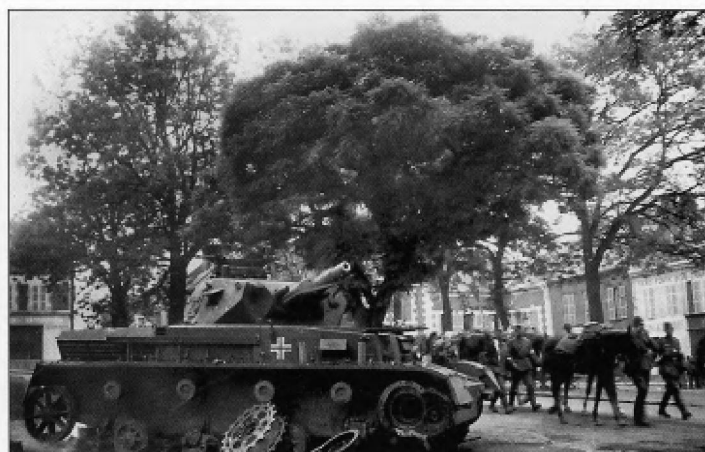
This severely damaged Pz.Kpfw.IV Ausf.C appears to have been cannibalized for spare parts and left abandoned in a French town. The drive sprocket and final drive housing has been removed and can be seen lying on the ground in front of the vehicle.
