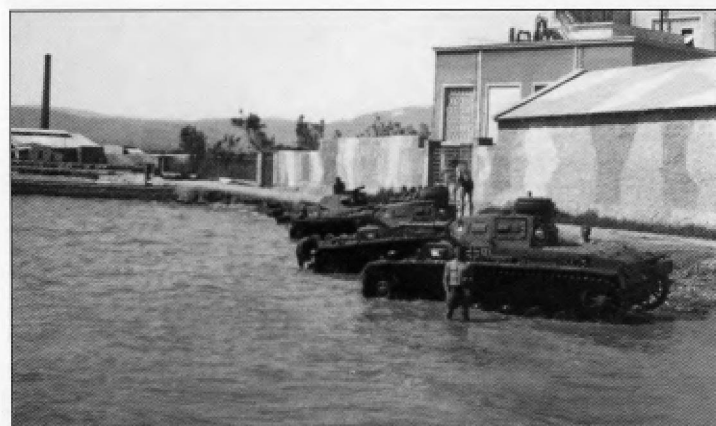
The crewmen of two Pz.Kpfw.III Ausf.H and a Pz.Kpfw.II from 2.Panzer-Division wash their dusty Panzers in a seaside town in the Balkans. The single rear plate of the new turret design can be seen here. After the campaign was over, the crews of this unit painted large playing card emblems on the sides and back of their tank turrets, like this white spade inside a white circle. An oversized white outline Balkenkreuz is also painted on the rear of the turret and the tactical number '121' is painted on the side of the hull behind the standard cross.
