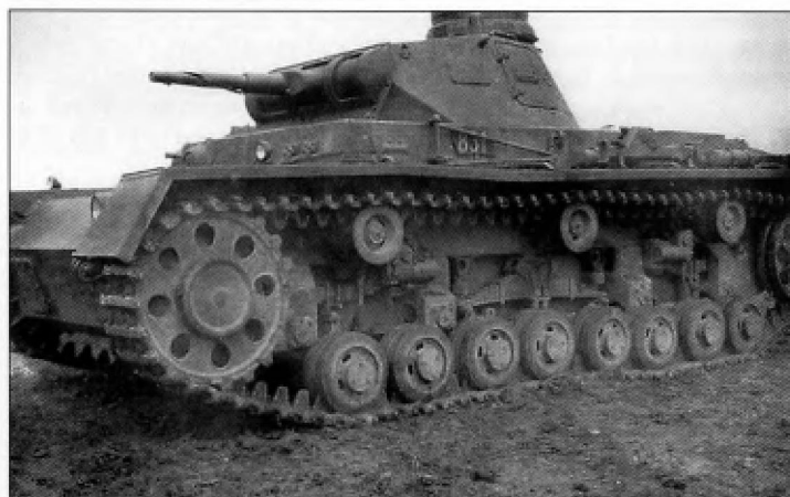
This photo of a Pz.Kpfw.III Ausf.C provides a good view of the eight wheel leaf spring suspension system. Note the egg shaped holes in the drive sprocket and the high guide teeth on the Kgs.6109/380/120 tracks. Also visible on the side of the hull is the swing arm used to mount an MG34 for use against ground attack aircraft by a crewman that was installed on the Pz.Kpfw.III Ausf. B-D.
