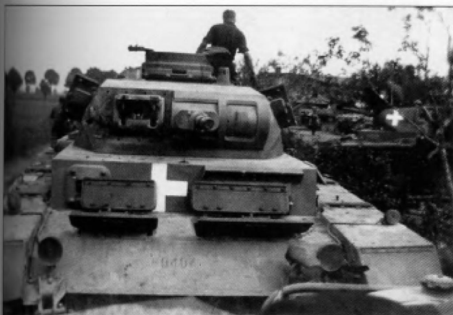
A Pz.Kpfw.III Ausf.E seen early in the Polish campaign, boldly marked with a large white Balkenkreuz on the front plate. The chassis number '60408' can be faintly seen on the front glacis plate making this the eighth Ausf.E produced. A hit on the front of the turret has torn away the right side of the external gun mantlet and made a small penetration hole in the 30mm armor plate. There were 96 Pz.Kpfw.III Ausf.E produced from December 1938 to October 1939.
