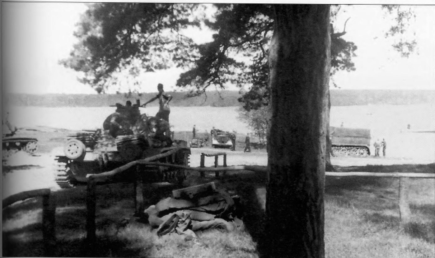
The deep wading exhaust fitted to this Pz.Kpfw.III Ausf.F or G converted to a Tauchpanzer can be seen in this rear view. A total of 168 Pz.Kpfw.III Ausf.F, G and H were converted to Tauchpanzer from July to October 1940.
