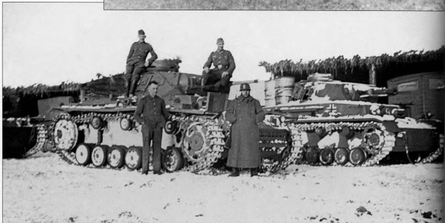
A Pz.Kpfw.III Ausf.J and a Pz.Kpfw.IV Ausf.F sit in a snow covered field in Russia during the winter of 1942-43. The short barrel 5cm KwK L/42 gun had proved to be inadequate against the Russian T-34 and KV tanks and would soon be replaced with the 5cm KwK L/60 gun.
