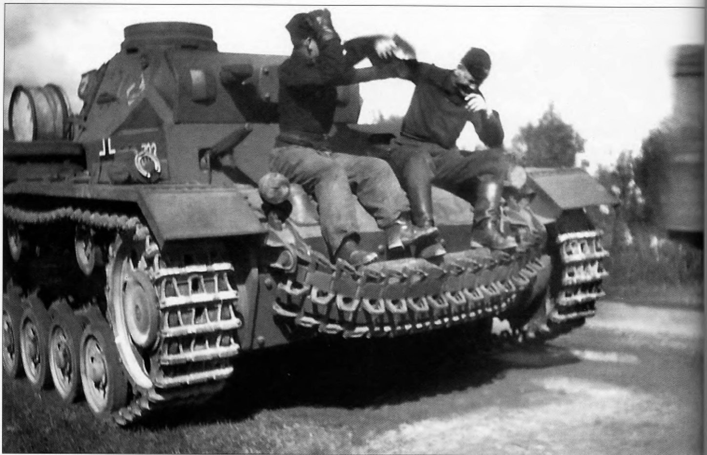
This Pz.Kpfw.III Ausf.F from 2.Panzer-Division has been rearmed with a 5cm KwK L/42 gun and upgraded with additional 30mm armor plates bolted to the lower hull on the front and rear and welded to the front superstructure plate. Due to the increased weight, the suspension was modified by the addition of 95mm wide rubber tired road wheels to replace the earlier 75mm wide tires and new 40 cm Kgs.61/400/120 tracks were fitted. Note the two types of track links. The ones stowed on the front have been redesigned with a slot on the outside edge to attach an ice sprag. Spacer rings were added to the drive sprocket and idler to accommodate the new tracks. The earlier cupola has been retained.
