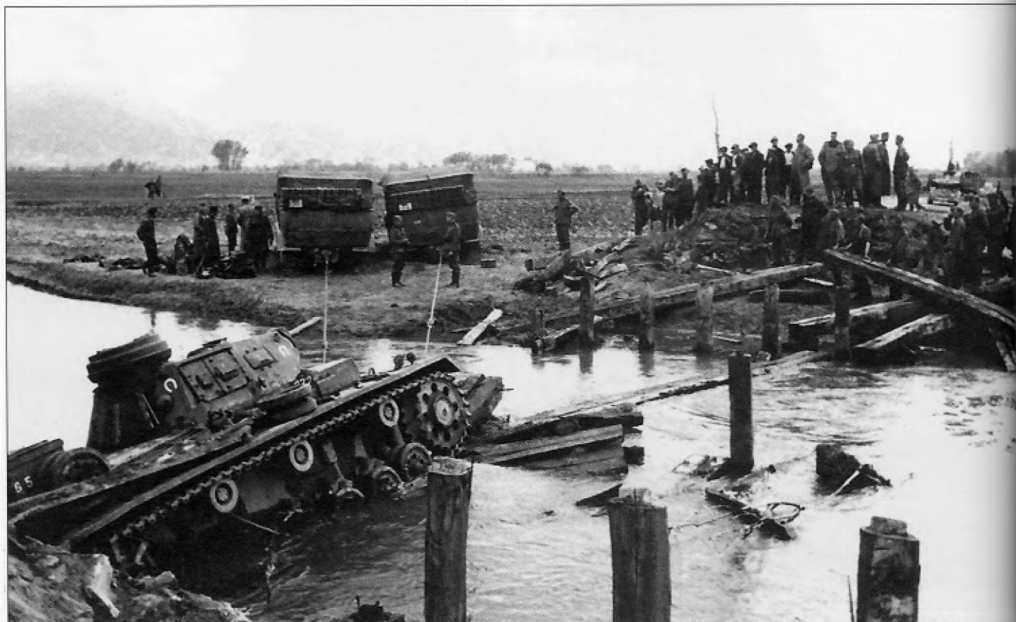
This Pz.Kpfw.III Ausf.G from 2.Panzer-Division has fallen through a wooden bridge somewhere in the Balkans in spite of having two good luck horseshoes attached to the turret, and is being towed out by two Sd.Kfz.9 half-track prime movers. It is fitted with a new cupola, turret ventilator and 95mm wide rubber-tired road wheels but still has the early 38cm tracks. The front return roller has been relocated forward.
