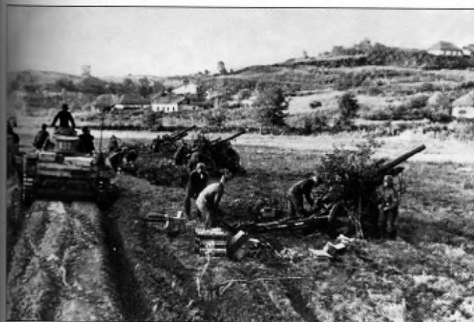
A Pz.Kpfw.III Ausf.G identified by the top hinged starter crank port cover and early cupola, rolls past a battery of 10.5cm leFH18 guns. The vehicle has also been fitted with a stowage bin on the rear of the turret and a smoke candle rack on the rear plate of the superstructure.
