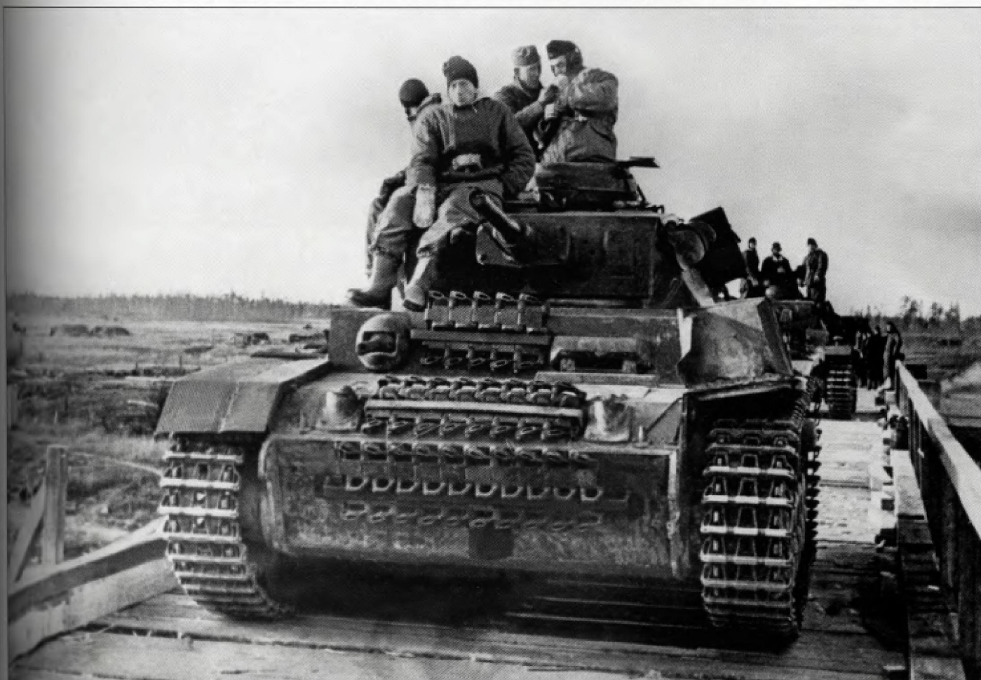
On the Pz.Kpfw.III Ausf.J, a single 50mm thick armor plate replaced the two 30mm plates used on the Pz.Kpfw.III Ausf.H on the front of the superstructure and lower hull. The thickness of the mantlet was increased from 35mm to 50mm as well while the front of the turret remained at 30mm. An improved driver's visor, the Fahrersehklappe 50 to fit the new 50mm front plate was also installed.
