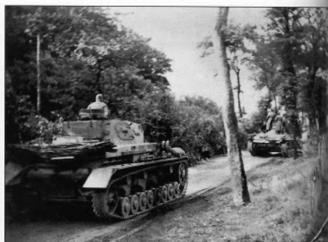
A Pz.Kpfw.IV Ausf.D, identified by the shape of the engine ventilation grille, rolls down a country road in France in May 1940. A non-standard turret stowage bin has been added to the turret and a large bundle of fascines and some personal belongings are being carried on the engine deck.
