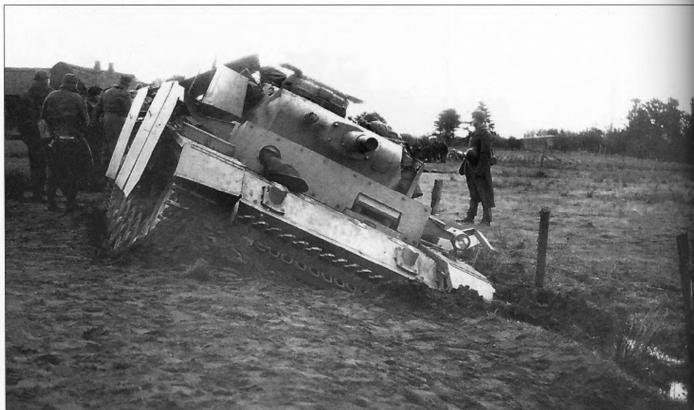
A Pz.Kpfw.III Ausf.N has gotten itself thoroughly mired in the soft ground beside a dirt road. This is one of 213 Pz.Kpfw.III Ausf.N manufactured on new Ausf. chassis as can be determined by the lack of headlight mounts beside the armored brake cooling vents. It was armed with the 7.5cm KwK L/24 which was more potent gun than the 5cm KwK L/60 gun. The two front hull Schürzen rail supports are of the style normally seen in the center position.
