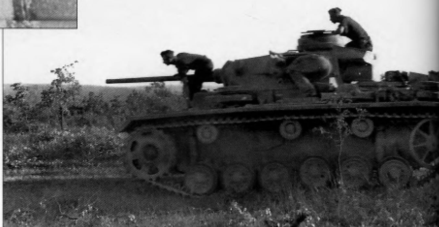
A Pz.Kpfw.III Ausf.J speeds along a dirt track in Russia during the summer of 1942. It was uncommon to see a Panzer III with the hub cap missing from the drive sprocket while it was quite common to see later production StuG.III Ausf.G without them.
