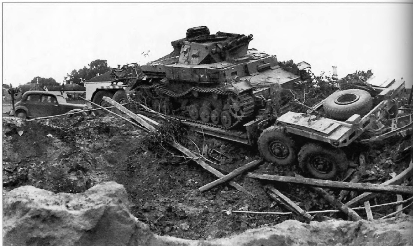
This Pz.Kpfw.IV Ausf.E has come to grief a second time when the Sd.Ah.116 trailer it was on fell into a bomb crater. A new, reinforced cupola was introduced on the Ausf.E along with a new pivoting driver's visor called the Fahrersehklappe 30. The rear plate on the turret was changed to a single bent plate which eliminated the bulge below the cupola and a new fume extraction fan was installed on the turret roof. The tactical number '200' can be seen painted in white on the side of the turret and a white outline rhomboid with a '2' beside it can be seen on the top left corner of the front plate.
