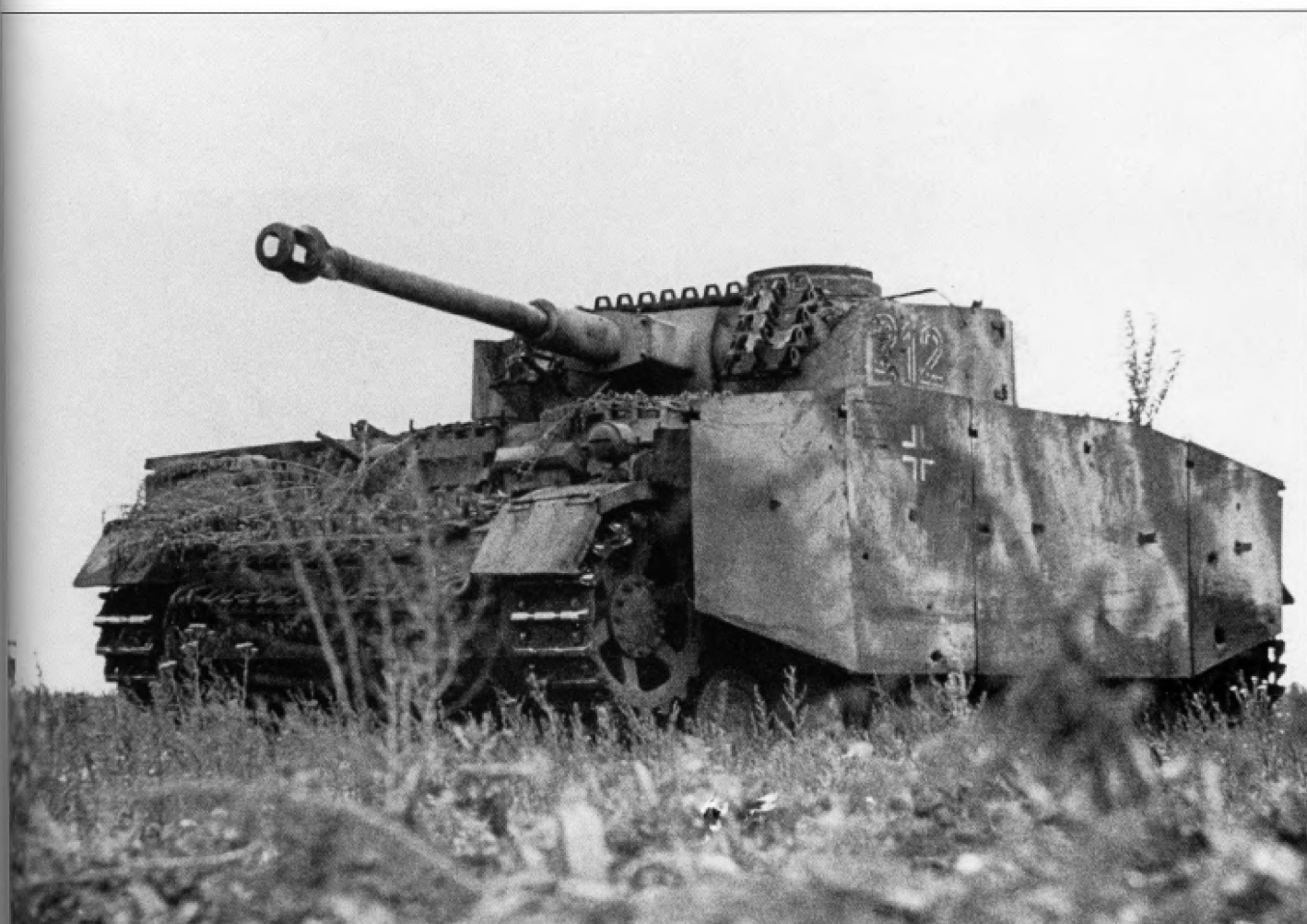
The early style of hull Schürzen was attached using hooks welded to a steel angle frame that ran down the side of the hull with additional hooks bolted to the fenders. Holes were cut into the plates for the hooks to go through. This arrangement often resulted in damage or loss of the skirts when snagged on brush and was changed to a saw-toothed early during production of the Ausf.H. A shipping stencil can be seen painted on the Schürzen just in front of the white outline Balkenkreuz.
