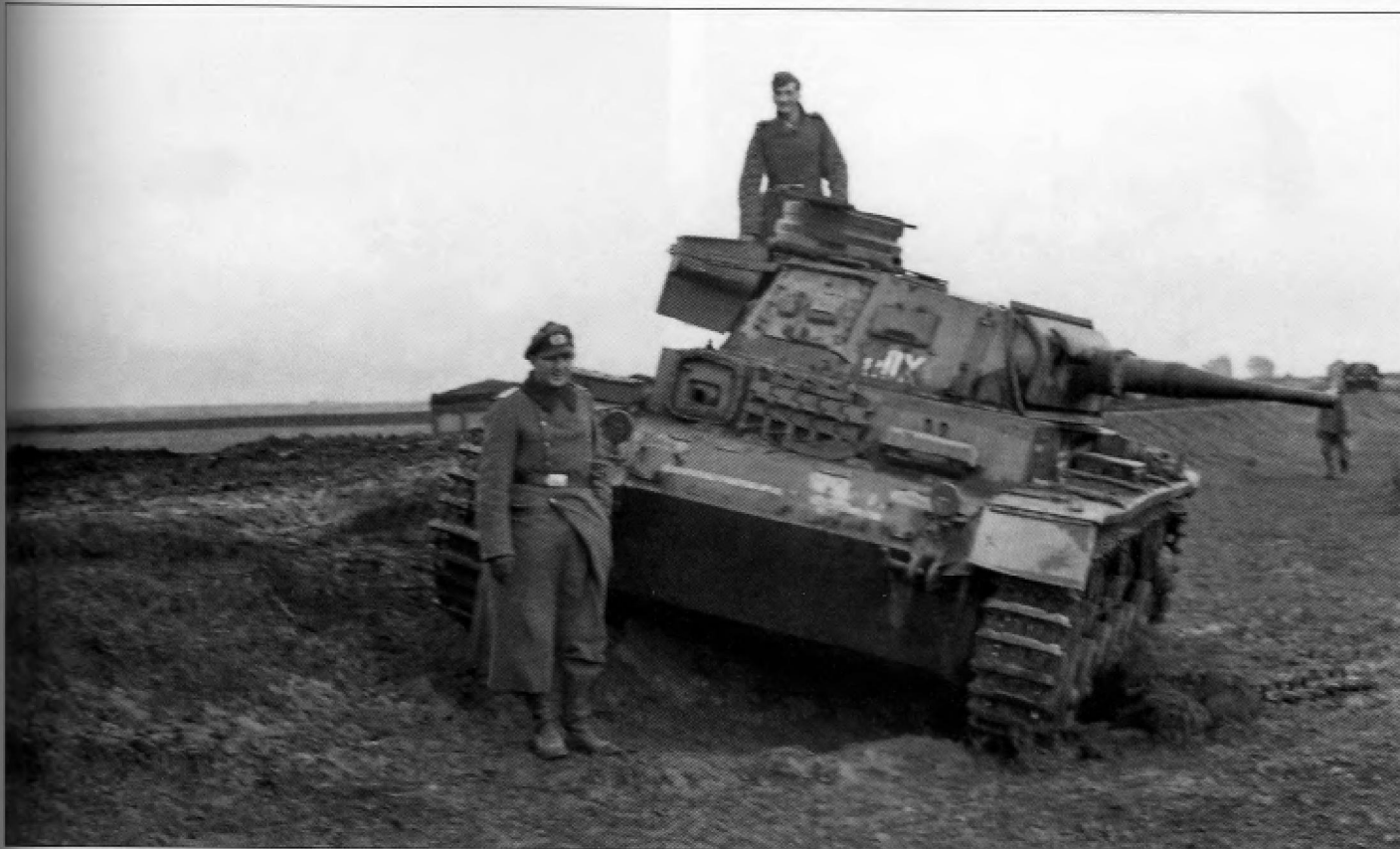
A later Pz.Kpfw.III Ausf.G converted to a Tauchpanzer that has been fitted with the 5cm KwK L/42 gun. The function of the steel strap attached to the front side of the turret by the lifting hook bolts is unknown. (Photo courtesy of John Prigent)
