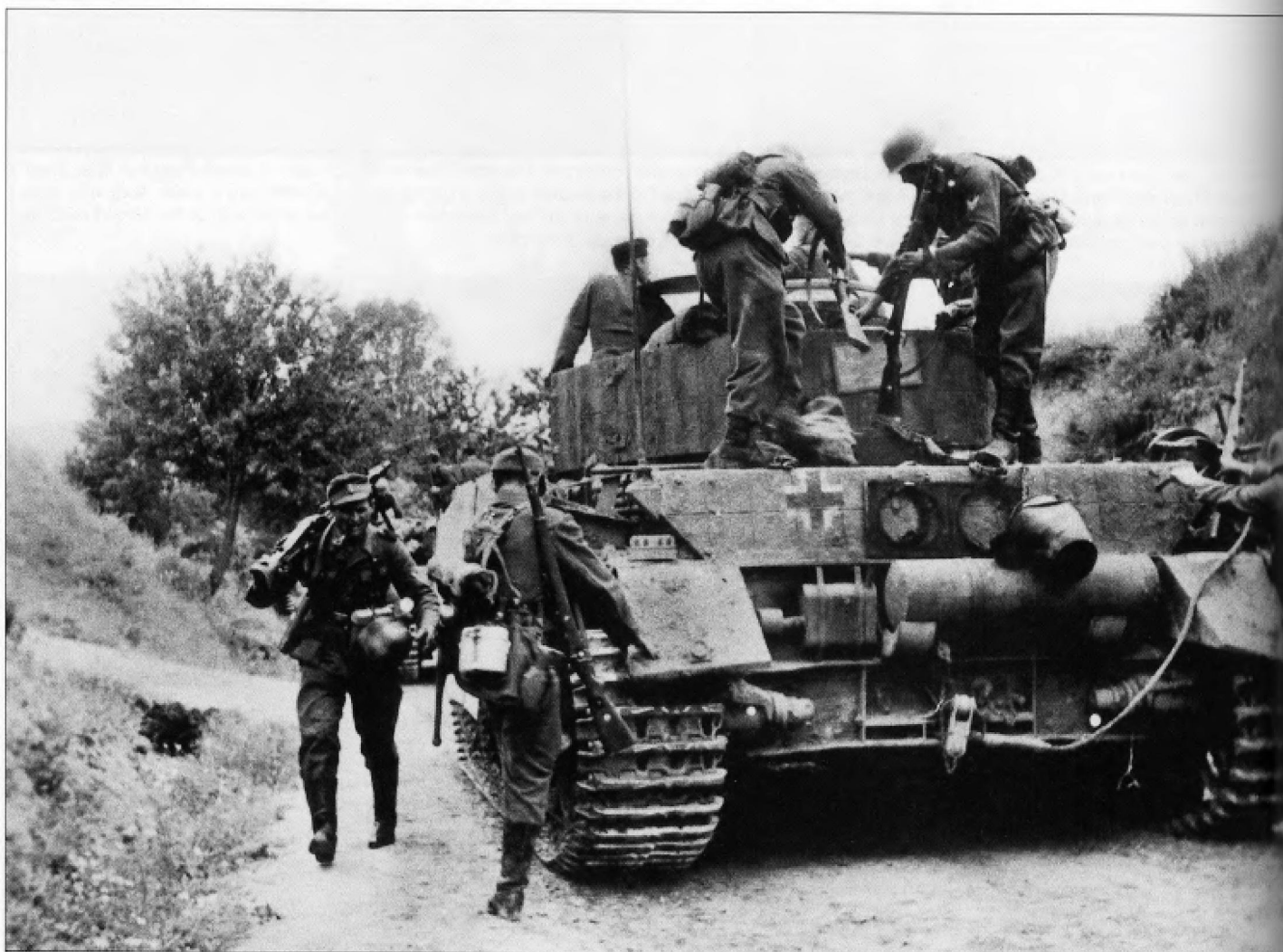
An early Pz.Kpfw.IV Ausf.H from Pz.Rgt.35 of the 4.Panzer-Division in Russia during the summer of 1944. The hull and turret Schürzen have been covered with a field workshop applied coat of Zimmerit with a unique herringbone pattern. It is fitted with the wider 'Ostkette' tracks that were issued only to units on the Eastern Front in May 1944.
